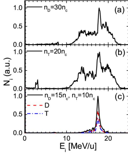
Fig.1. (Color online) Ion energy spectra at  $t = 100\tau$  from PIC simulations. The laser amplitude is  $a = 50$  and targets are: (a) deuterium target with  $n_e = n_D = 30n_c$ , (b) tritium target with  $n_e = n_T = 20n_c$ , and (c) DT target with  $n_D = 15n_c$ ,  $n_T = 10n_c$ , and  $n_e = 25n_c$ . The respective spectra for deuterons (red dashed) and tritons (blue dash-dotted) from the DT target are also drawn in (c).
