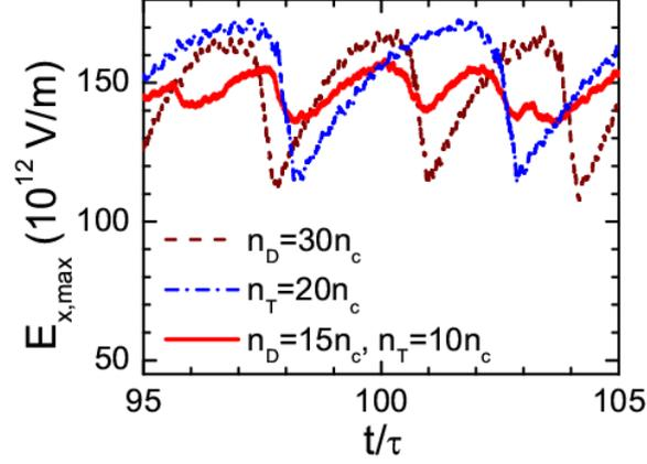
Fig.4. (Color online) Time evolution of the magnitude of the longitudinal electric field  $E_{x,\max}$  in three different targets, the laser and target parameters are the same as in figure 1.
