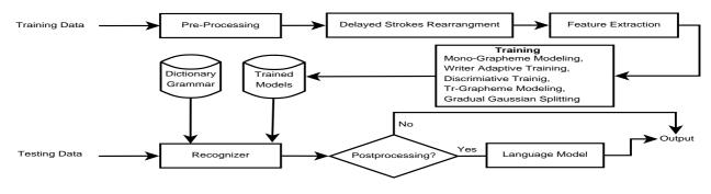
Figure 1. Block Diagram
