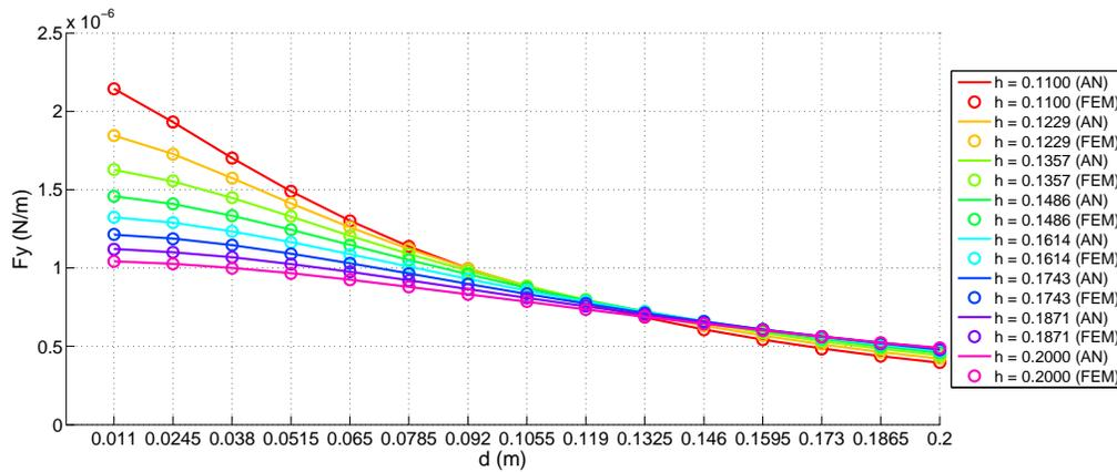
Figure 6: y-component of the force for adjacent massive conductors.  $a = 0.005$  m,  $b = 0.05$  m
