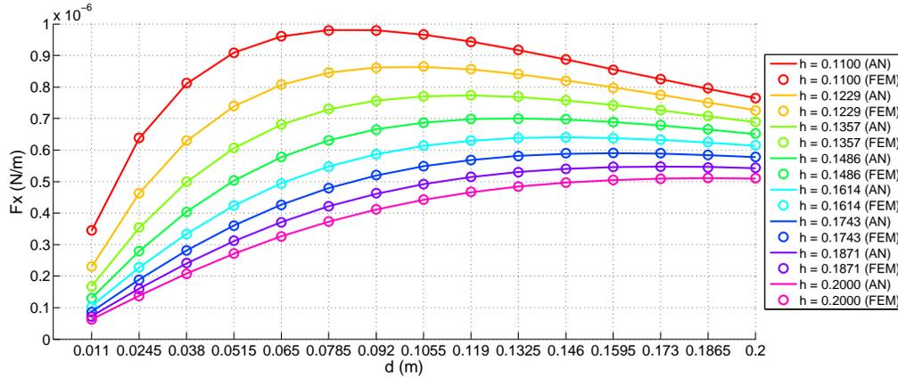
Figure 5: x-component of the force for adjacent massive conductors.  $a = 0.005$  m,  $b = 0.05$  m
