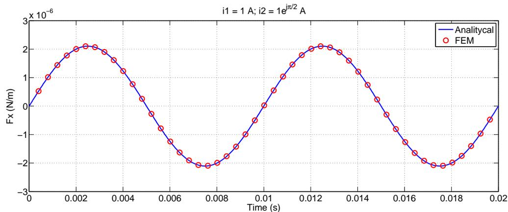
Figure 4: x-component of the force for adjacent massive conductors.  $a = 0.005$  m,  $b = 0.05$  m
