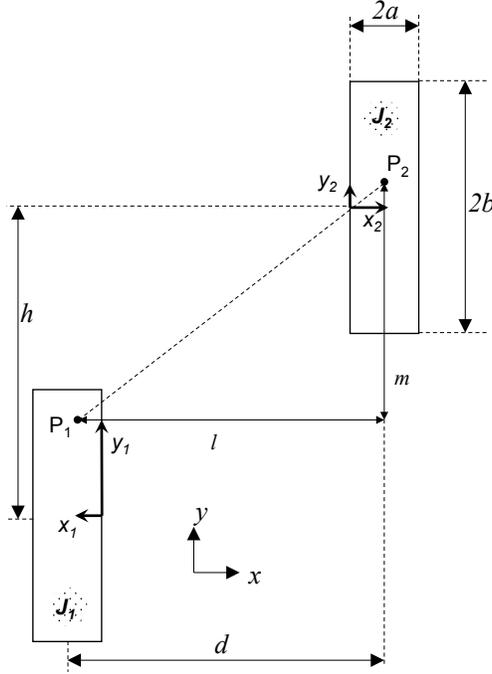
Figure 1: Layout of non-adjacent massive conductors.
