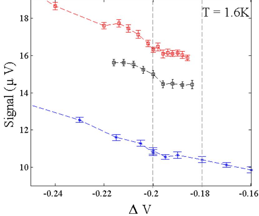
Figure 3: Plot of electron signal left above  $T_4$  after multiple splitting of electron packets, versus  $\Delta V$ , the voltage difference between  $T_2$  and  $T_4$ . A plateau is seen in the region between  $\Delta V = -0.20\text{V}$  to  $-0.18\text{V}$ . 1V change on the  $T_2$  gate corresponds to changing the potential on the helium surface by approximately 20meV. Each dataset is from a different experiment. Dotted lines connecting data points are guide to the eye.
