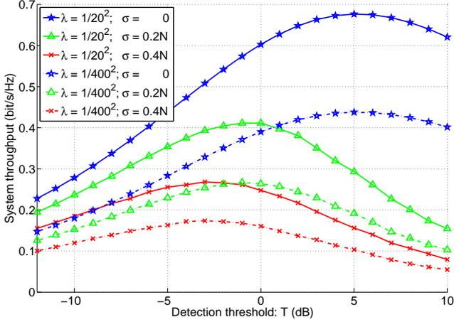
Fig. 9. System throughput versus detection threshold.
