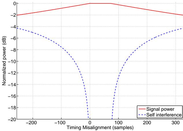
Fig. 2. Signal and self-interference powers of an OFDM signal received on the central subcarrier with timing misalignment.  $N = 1024$ ;  $N_{cp} = 72$ ; the used subcarriers are  $\{-300, \dots, 0, \dots, 299\}$ .
