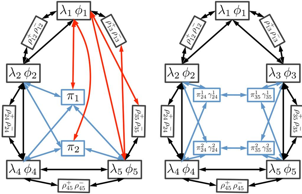
Fig. 3: Communication requirements for the power network in Fig. 2 when bus 3 has no injection as described in Section VI-A (left), and for the distributed inter-area flow constraint formulation of Section VI-B (right).
