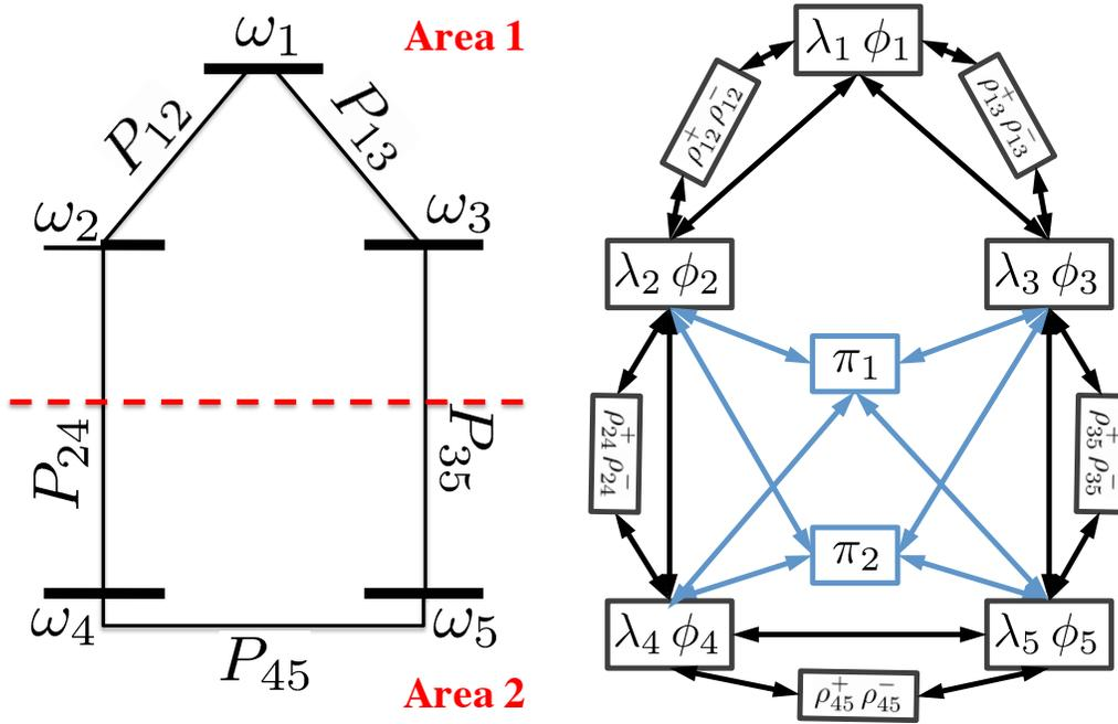
Fig. 2: Power network example (left) and the corresponding communication requirement to implement the distributed load control (18)
