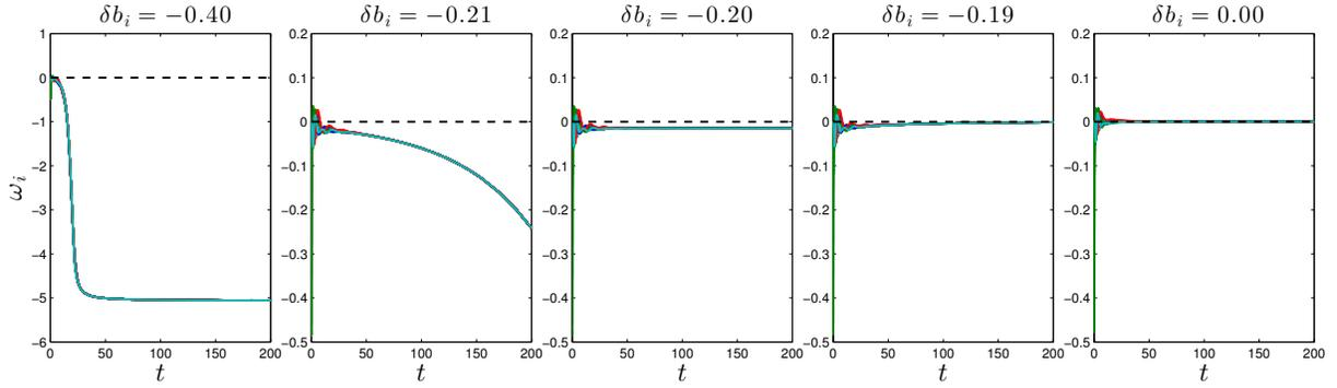
Fig. 10: Bus frequency evolution for homogeneous perturbation  $\delta a_i \in \{-0.4, -0.21, -0.2, -0.19, 0.0\}$
