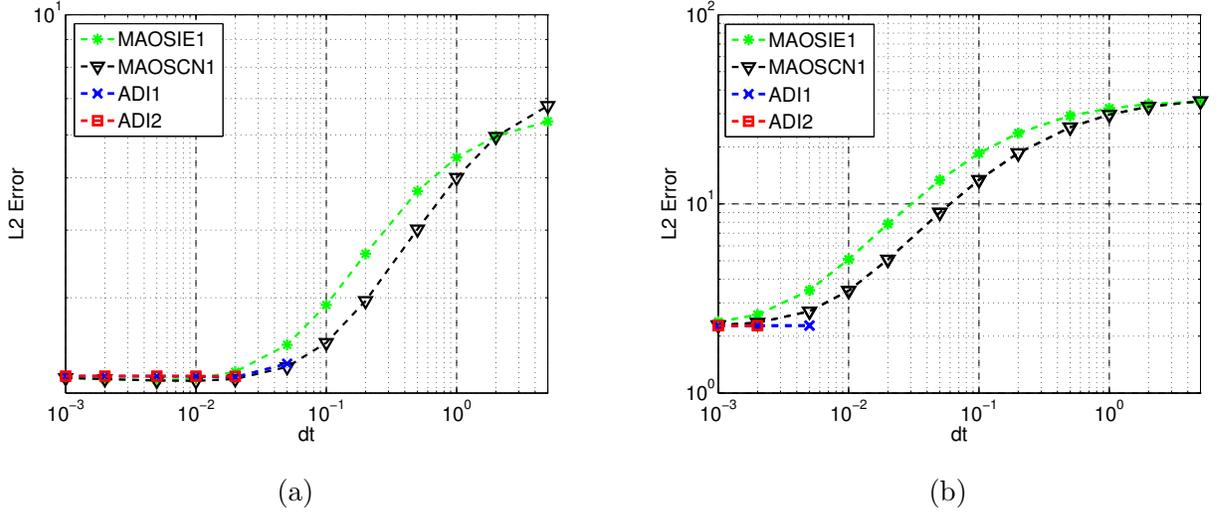
Figure 3: Stability verification of the MAOS and ADI schemes with  $H = 1$ . (a)  $h = 0.5$ ; (b)  $h = 0.25$ .
