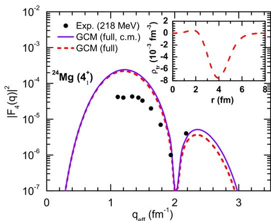
FIG. 7: (color online) Longitudinal C4 form factor  $|F_4(q)|^2$  for the transition from the ground state to the  $4_1^+$  state of  $^{24}\text{Mg}$ , in comparison with available data. The inset shows the corresponding transition density. Data are taken from Ref. [91].
