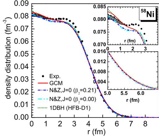
FIG. 11: (color online) Comparison between the charge distribution of the ground state of  $^{58}\text{Ni}$  obtained using single projected mean-field configurations or the full GCM basis and the experimental data [100]. A previous calculation using a one-dimensional Bohr Hamiltonian based on an HFB calculation with the Gogny D1 force (1DBH) [101] is also shown. The insets magnify the profile of the charge density at very small radii and in the nuclear surface.
