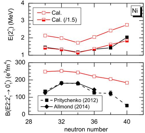
FIG. 14: (color online) The excitation energy  $E(2_1^+)$  of  $2_1^+$  state and the  $B(E2)$  value for the transition from this state to the ground state for  $^{58-68}\text{Ni}$ . Experimental data are taken from Refs. [94, 102].
