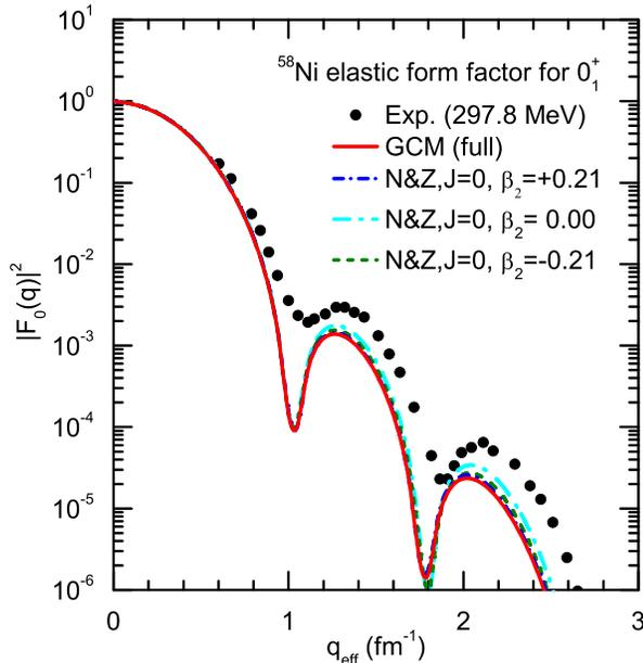
FIG. 10: (color online) Data for the elastic form factor  $|F_0(q)|^2$  for the ground state of  $^{58}\text{Ni}$  taken from Ref. [99] in comparison with the form factor obtained from four different calculations: projection of a single HFB configuration with either  $\beta_2 = 0$  (spherical shape) or  $\beta_2 = \mp 0.21$  (oblate and prolate minima of the  $J = 0$  energy curve) and full GCM of projected states.
