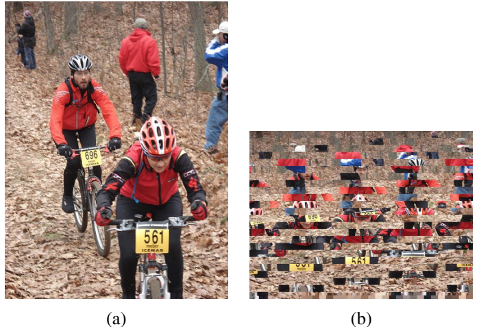
Fig. 1. An image from PASCAL VOC2010 is decoded with wrong width. (a) The original image 2007_001630.jpg with width 375. (b) The image is decoded with the wrong width 512.
