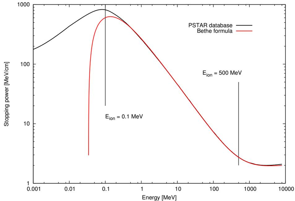
Figure 1.2. Stopping power of protons in liquid water based on PSTAR database [Berger et al., 2005] and on the Bethe formula 1.2, implemented in the libamtrack library. The range of ion energies (0.1 – 500 MeV) relevant to ion radiotherapy is shown by vertical lines
