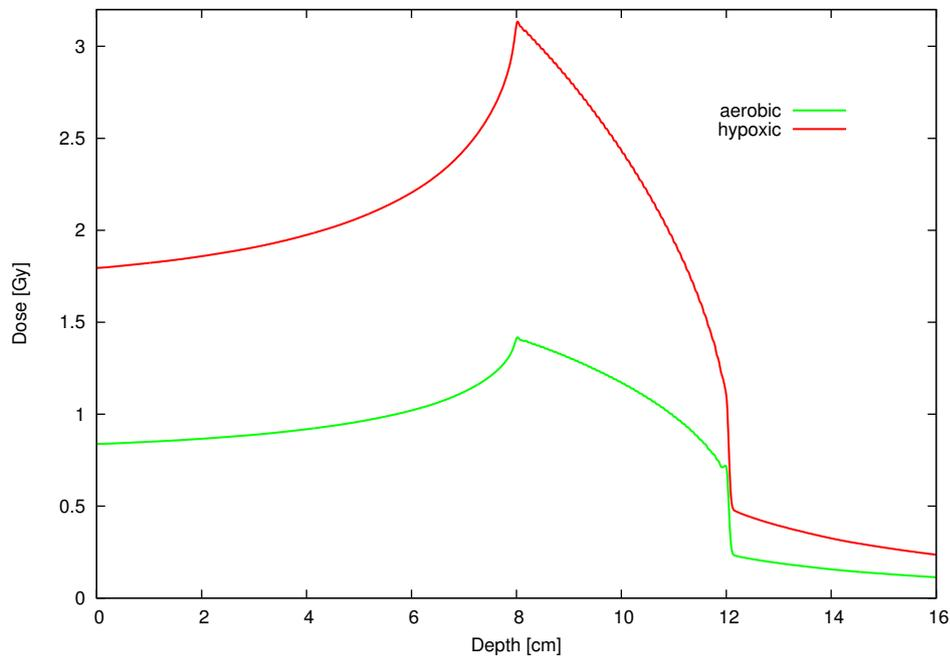
Figure 5.9. Dose depth-profiles related to cell survival profiles presented on figure 5.8. Calculations performed using the libamtrack library.
