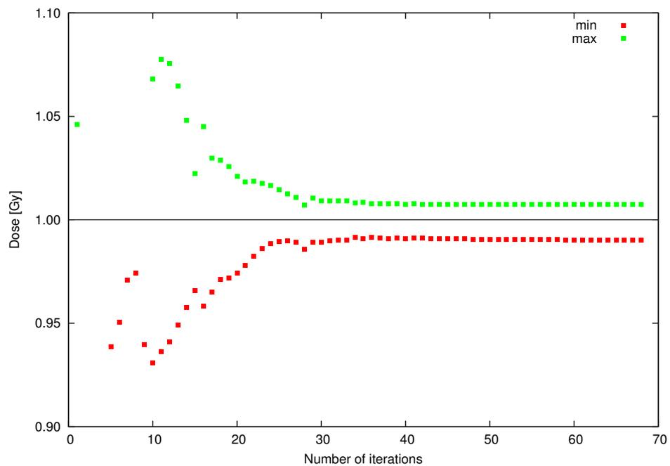
Figure 4.6. Convergence of the dose profile optimization algorithm. Points show the minimum and maximum dose values over the depth of the flat region (8-12 cm) after each iteration step. Calculations performed using the libamtrack library
