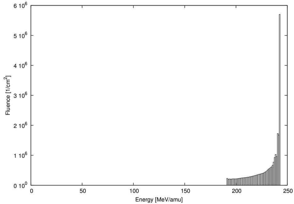
Figure 4.5. Initial energies and fluences of the 49 carbon ion beams required to achieve the flat dose profile presented in the upper panel of Fig. 4.4. Each bar corresponds to a single pristine Bragg peak of initial energy given on the abscissa. Calculations performed using the libamtrack library.
