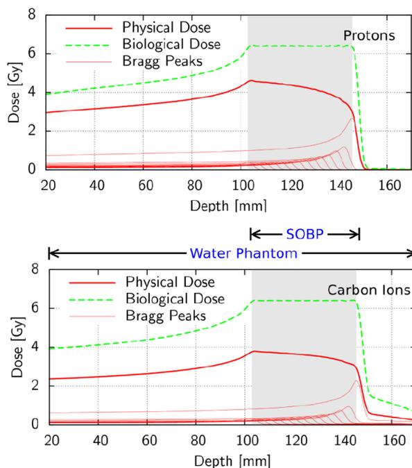
Figure 2. Illustration of depth distributions of “physical dose” (or of depth-dose) and of “biological dose” (or of depth-cellular inactivation level) in spread-out carbon and proton beams, in a water phantom. The spreading-out of the Bragg peak is achieved by a suitable superposition of ion beams of different initial energies and fluences. Reprinted from <http://totlxl.to.infn.it/>, Andrea Attili, INFN-TPS project resources.
