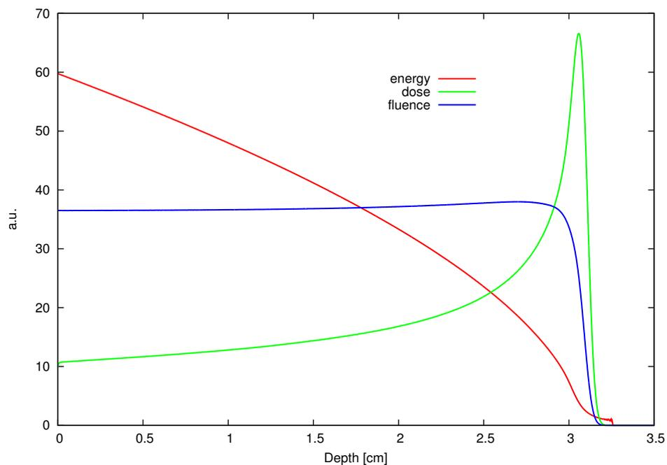
Figure 1.3. Depth-dose dependence, mean energy vs. depth, and fluence vs. depth of a pristine (non-modulated) proton beam. The entrance values (at 0 cm depth) are: energy:  $E = 59.75$  MeV; dose:  $D = 1.727$  Gy; and fluence:  $F = 10^9$  ions/cm<sup>2</sup>. Calculations made by the author, using the Geant4 package and the libamtrack library.
