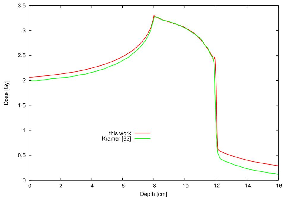
Figure 5.5. The depth-dose profile used in calculation of Kramer and Scholz [Krämer and Scholz, 2000] (green line) compared with depth dose profile calculated with the aid of the libamtrack library (red line). Profile marked with red line was adjusted to agree with Kramer's profile in depths range between 8 and 12 cm. Calculations performed using the libamtrack library.
