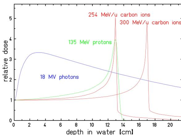
Figure 1. Relative depth-dose profiles of photons, protons and carbon ions. The Bragg peak of proton and carbon beams is clearly visible. Note that all dose profiles have been normalized to the same entrance dose. Reprinted from Haettner [Haettner, 2006].
