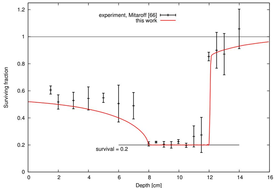
Figure 5.4. Survival of CHO cells vs depth: results of calculations using the survival optimization algorithm and the scaled Katz model, where CHO cells are represented by the model parameters:  $m = 2.31$ ,  $D_0 = 1.69$  Gy,  $\sigma_0 = 5.96 \cdot 10^{-11} \text{ m}^2$ , and  $\kappa = 1692.8$  (cf. Fig. 5.1, lower panel), calculations performed using the libamtrack library, compared with experimental data published by Mitaroff et al. [Mitaroff et al., 1998].
