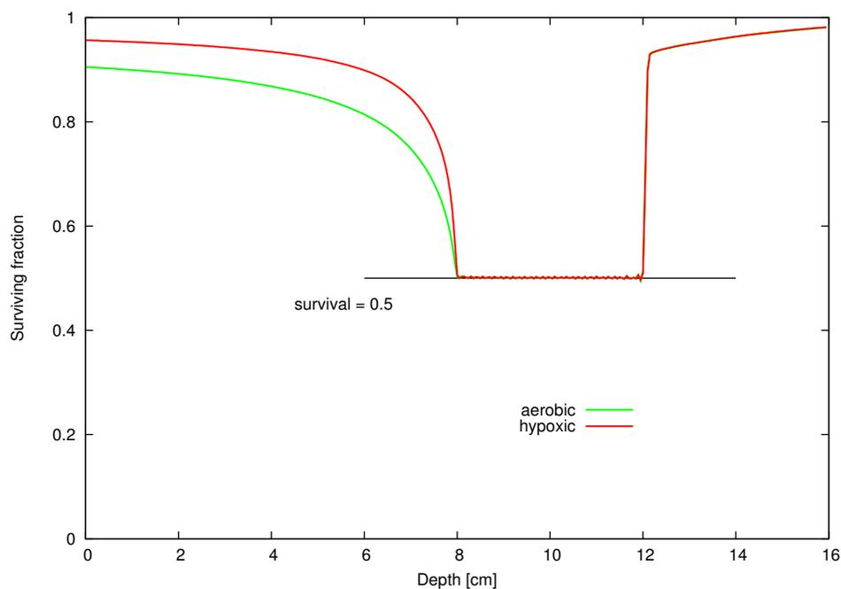
Figure 5.8. Cell survival depth-profiles calculated for aerobic and hypoxic V79 cells using Katz model (parameters listed in Table 5.2). For each case: aerobic and hypoxic two different beam configurations were used, each prepared in such way that the designed survival was equal to 0.5 over the interval between 8 and 12 cm. Calculations performed using the libamtrack library.
