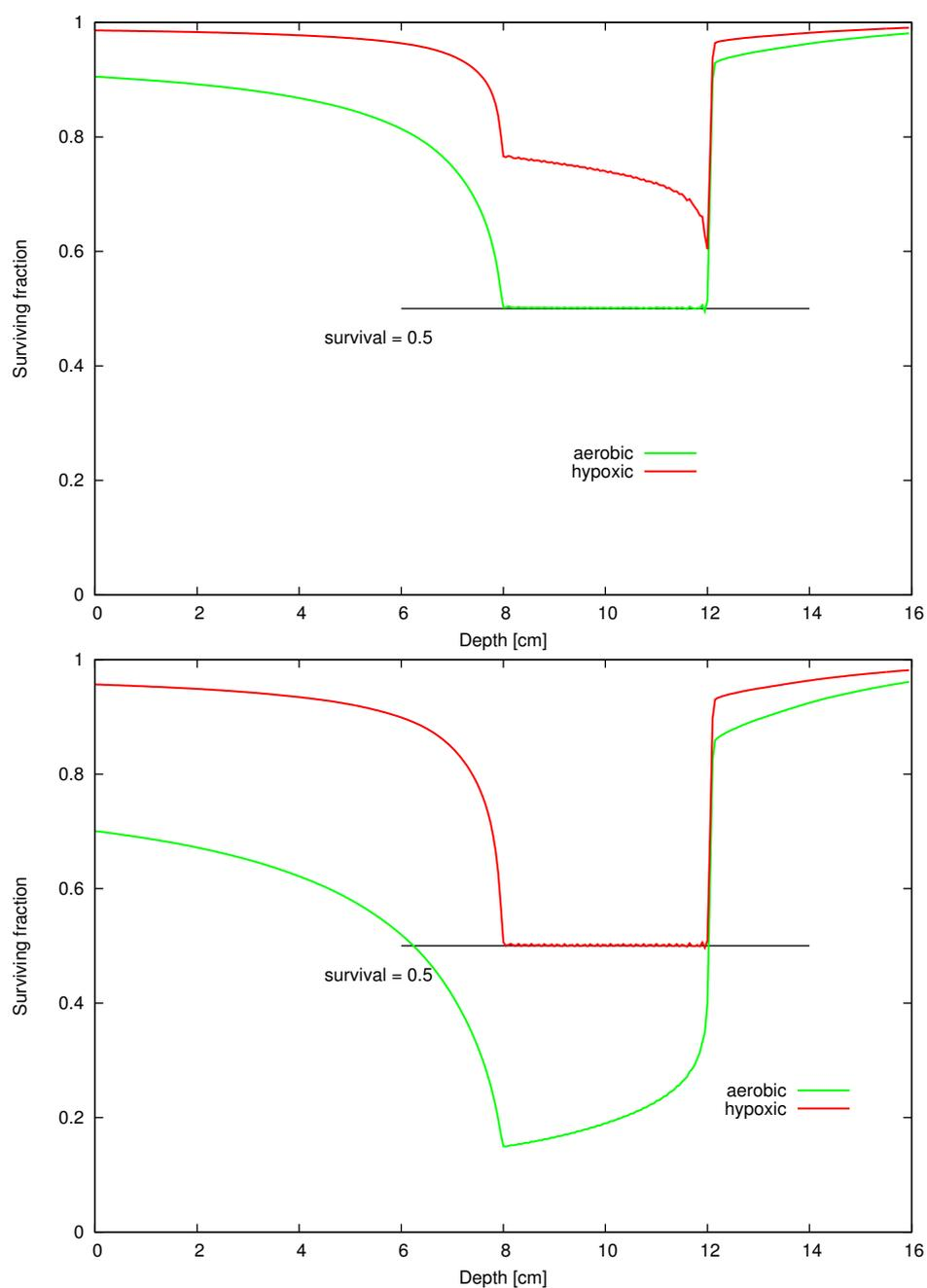
Figure 5.11. Cell survival depth-profiles calculated for aerobic and hypoxic V79 cells in two identical carbon ion beams. Initial beam configuration was prepared for the survival of hypoxic cells to be 50% (0.5) over the target region between 8 and 12 cm.
