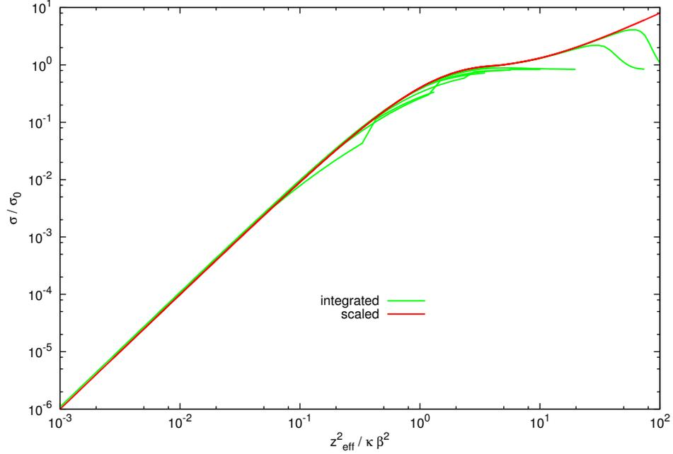
Figure 3.3. Inactivation cross-sections, normalised to  $\sigma_0$  vs.  $z^{*2}/\kappa\beta^2$ , based on the radial dose distribution function of Zhang. Calculations were performed using the integration (green lines) and scaled (red lines) versions of the Katz model, for ions of  $Z=1,2,3,5,10,50$  and  $100$  and energies  $0.1 - 500$  MeV/amu. Katz model parameters used:  $m = 2$ ,  $D_0 = 5$  Gy,  $a_0 = 1 \mu\text{m}$ ,  $\kappa = 2500$ ,  $\sigma_0 = 1.2 \pi a_0^2$
