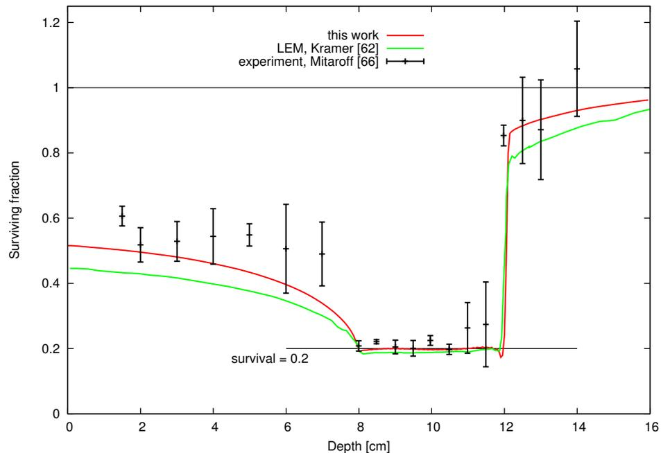
Figure 5.6. Survival of CHO cells vs depth: results of calculations using the dose optimization algorithm (dose profile presented on figure 5.5) and the scaled Katz model, where CHO cells are represented by the model parameters:  $m = 2.31$ ,  $D_0 = 1.69$  Gy,  $\sigma_0 = 5.96 \cdot 10^{-11}$  m<sup>2</sup>, and  $\kappa = 1692.8$ , calculations performed using the libamtrack library, compared with results of LEM calculations (reproduced from Kramer et al. [Krämer and Scholz, 2000]).
