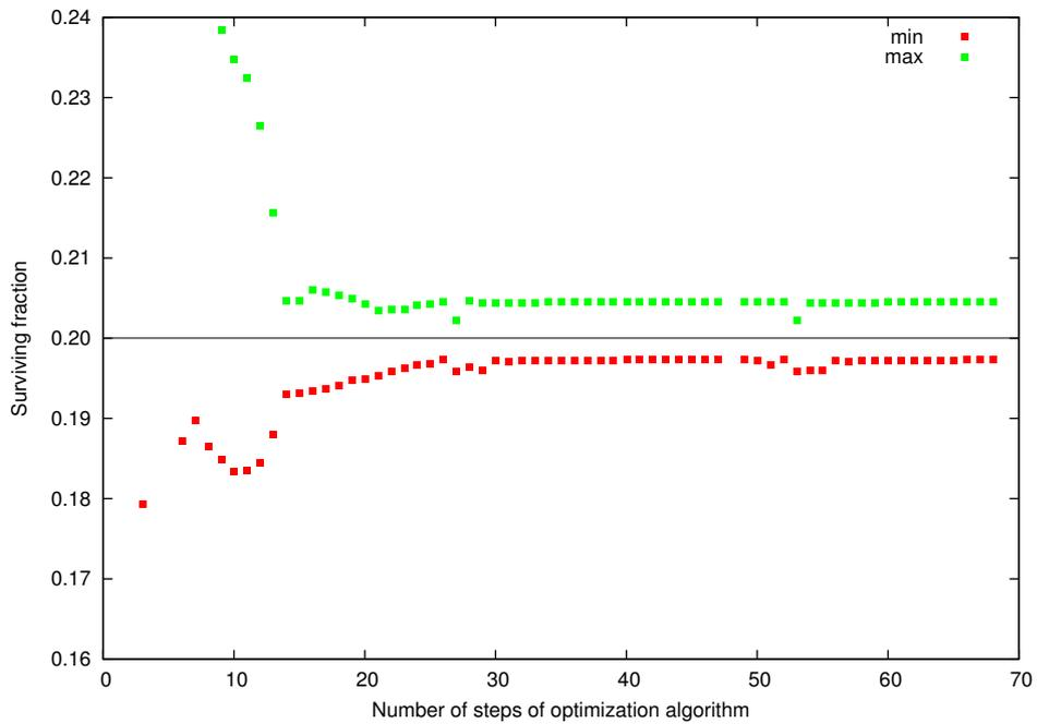
Figure 5.3. Convergence of the dose profile optimization algorithm. Points show the minimum and maximum dose values over the depth of the flat region (8-12 cm) after each iteration step. Calculations performed using the libamtrack library
