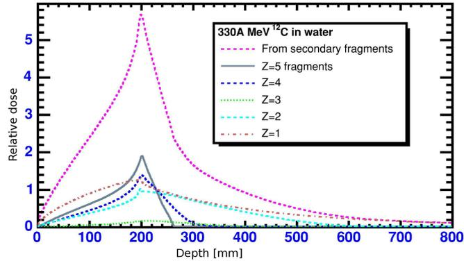
Figure 3. Monte Carlo-calculated contribution to the dose from secondary fragments of a 330 MeV/amu carbon ion in water. The nominal range of this monoenergetic carbon beam is 200 mm. Reprinted from Pshenichnov et al. [Pshenichnov et al., 2005]
