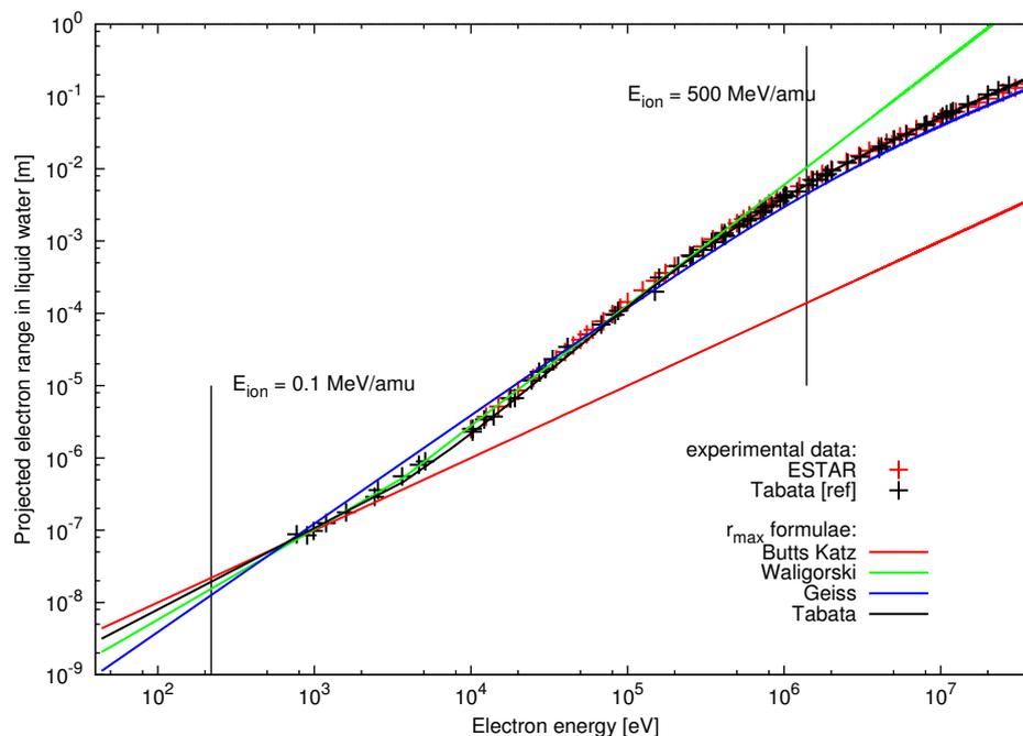
Figure 2.1. Projected electron ranges vs. initial electron energy in liquid water. Experimental data are from Tabata [Tabata et al., 1972] (measurements in different materials, density-rescaled to liquid water). The ion energy range useful in ion beam radiotherapy is indicated by vertical lines. Experimental data and the respective electron energy-range relationships have been implemented in the libamtrack library.
