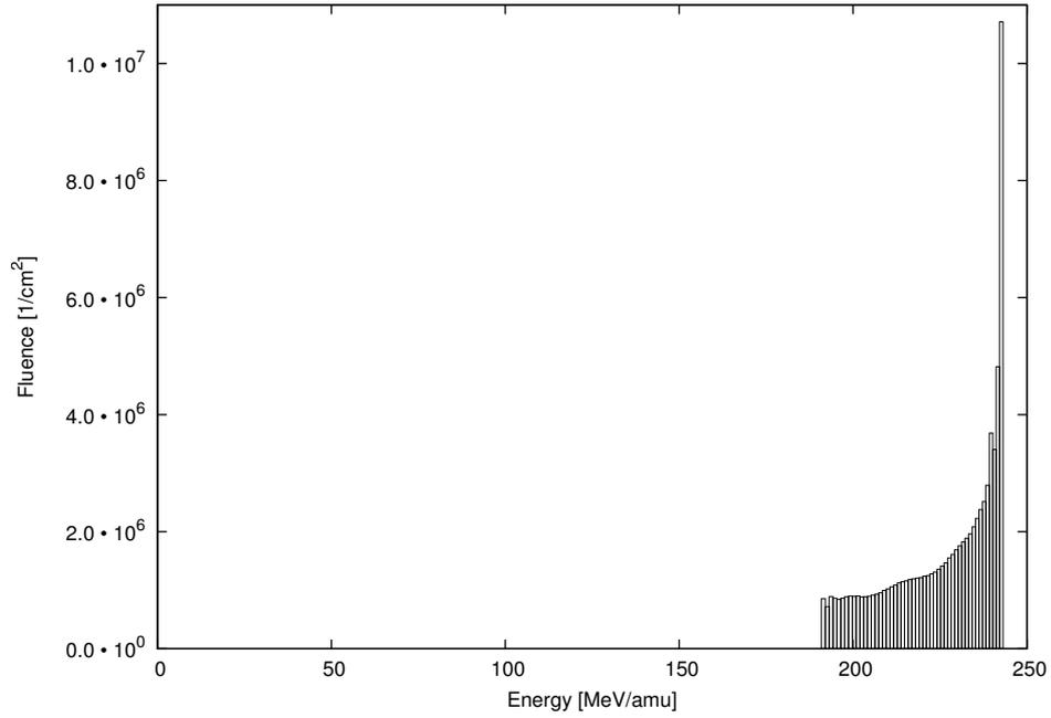
Figure 5.2. Initial energies and fluences of the 49 carbon ion beams required to achieve the flat survival profile presented in the upper panel of Fig. 5.1. Each bar corresponds to a single pristine Bragg peak of initial energy given on the abscissa. Calculations performed in liquid water, using the libamtrack library.
