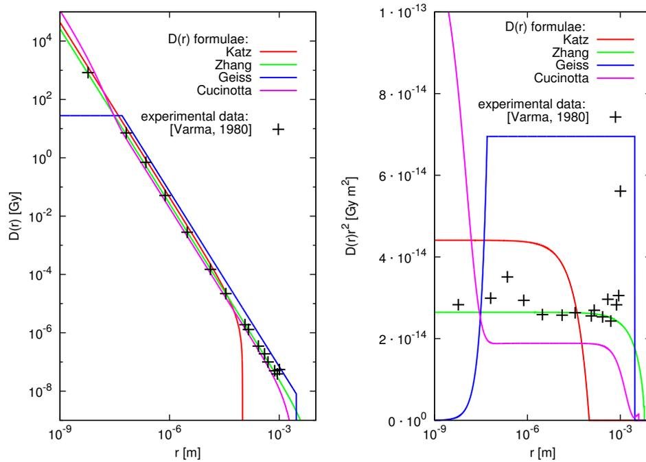
Figure 2.2. Comparison of experimentally measured radial distribution of dose around 377 MeV/amu neon ions in tissue-equivalent gas [Varma and Baum, 1980] and  $D(r)$  calculated using the formulae of Katz, Zhang, Geiss and Cucinotta. Experimental uncertainties were not provided by Varma et. al. The right-hand panel shows the same data and calculations, but on a semi-logarithmic plot where data points and results of  $D(r)$  calculations are multiplied by their respective  $r^2$  values.
