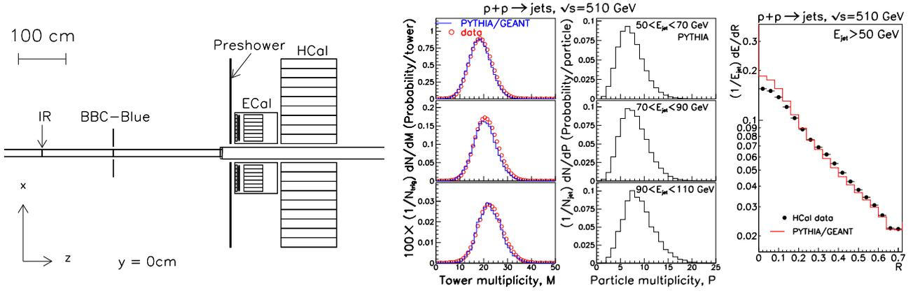
**Figure 9.** (left) Schematic of apparatus used for  $p^{\dagger}p \rightarrow \text{jet}+X$  [47]; (middle) multiplicities from the anti- $k_T$  jet-finding algorithm for (left panel) the HCal response in data and full simulation and (right panel) for particles as generated by PYTHIA [53]; (right) distribution of energy with respect to jet axis.
