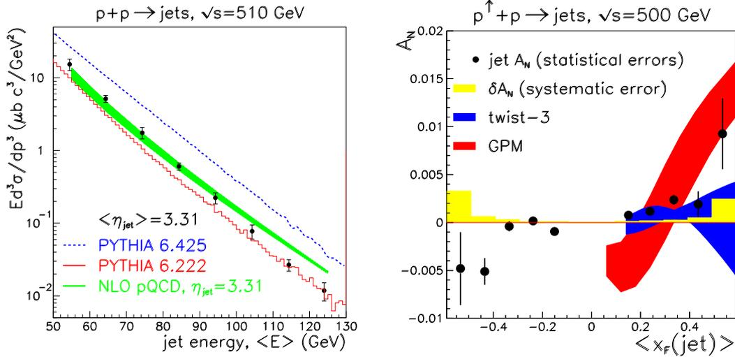
**Figure 11.** (left) Cross section for forward jet production in  $pp$  collisions at  $\sqrt{s} = 510$  GeV, in comparison to NLO pQCD and PYTHIA; (right)  $A_N$  for forward jet production, in comparison to calculations that fit the Siverts effect for SIDIS.
