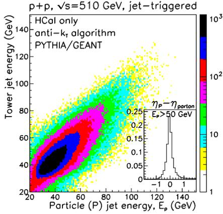
**Figure 10.** Comparison of results from the anti- $k_T$  algorithm applied to full PYTHIA + GEANT simulations versus events generated by PYTHIA [53]. The inset shows the directional match between particle jets and hard-scattered partons, and results in an 82% match when  $|\Delta\eta|, |\Delta\phi| < 0.8$ .
