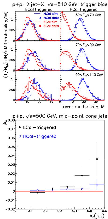
**Figure 12.** The impact of trigger bias is evident for mid-point cone jets reconstructed for events with an ECal trigger, corresponding to  $\sum E_{ECal} \geq 22$  GeV. (Top) tower multiplicity distributions show a bias towards jets with larger electromagnetic multiplicities for an ECal trigger; and (Bottom) the trigger bias makes jets more  $\pi^0$  like, thereby impacting their spin asymmetry.
