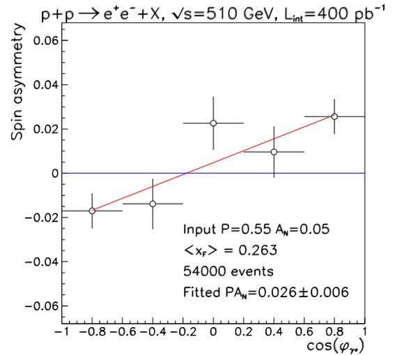
**Figure 13.** Projected sensitivity to  $A_N$  for DY production for a forward detection system proposed for installation at STAR in 2016.  $M_{\gamma^*} > 4$  GeV/c<sup>2</sup> is imposed, but otherwise DY kinematics match those from SIDIS [35, 36].
