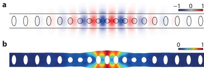
FIG. 5. **FEM simulations.** **a**, Electric field  $E_y$  component of the optical mode at frequency  $\omega_c/2\pi = 194$  THz (polarization in the plane of the page and transverse to the long axis of the nanobeam). **b** Displacement field of the mechanical breathing mode at frequency  $\omega_m/2\pi = 5.1$  GHz.
