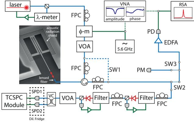
FIG. 6. **Experimental setup.** Phonon counting setup.  $\lambda$ -meter: wavemeter, FPC: fiber polarization controller,  $\phi$ -m: electro-optic phase modulator, VOA: variable optical attenuator, SW: optical switch, PM: optical power meter, EDFA: erbium-doped fiber amplifier, PD: fast photodiode, RSA: real-time spectrum analyzer, VNA: vector network analyzer, VC: variable coupler, SPD: superconducting single photon detector, TCSPC: time-correlated single photon counting.
