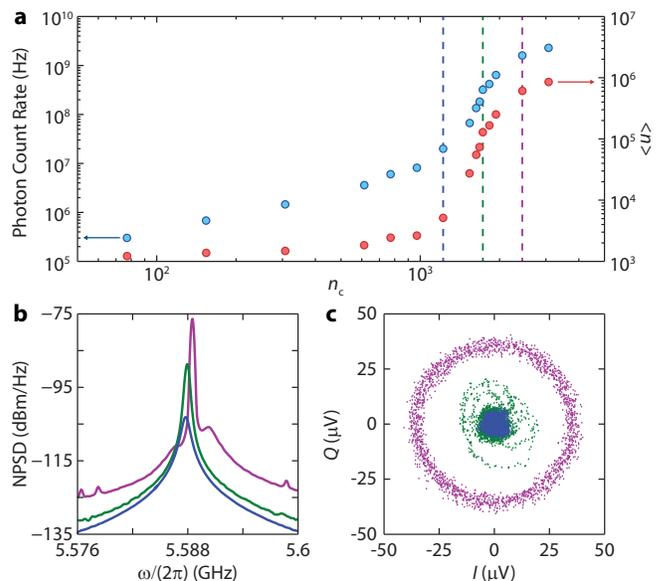
FIG. 3. **a**, Phonon count rate (blue) and inferred phonon occupancy  $\langle n \rangle$  (red) as a function of intracavity photon number for  $\Delta = -\omega_m$ . Dashed lines indicate points below (blue), at (green), and above (magenta) threshold. **b**, Noise power spectral densities (NPSD) corresponding to the dashed lines in **a**. **c**, Phase plots of the in-phase ( $I$ ) and in-quadrature ( $Q$ ) amplitudes of the detected optical noise corresponding to the dashed lines in **a**
