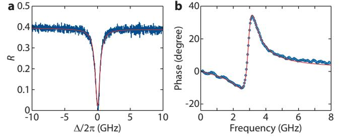
FIG. 7. **Optical cavity response.** **a**, Optical reflection spectrum of the cavity resonance versus cavity detuning  $\Delta = \omega_c - \omega_l$  (blue) with a Lorentzian fit (red) yielding  $Q_c = 236,000$ . **b**, Phase response of the optical resonance, yielding  $\kappa_e/\kappa = 0.52$ .
