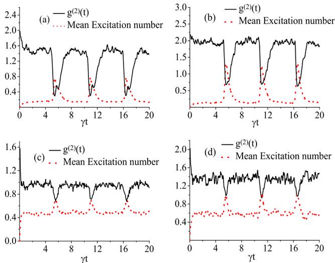
FIG. 4. Time-evolution of the averaged photon number and the second-order correlation function for two regimes of KNR. The parameters are: (a),(c)  $\Delta = 0$ ,  $\chi/\gamma = 15$ ,  $\Omega/\gamma = 6$ ; (b),(d)  $\Delta_2 = \omega_0 - \omega_2 = -\chi$ ,  $\chi/\gamma = 30$ ,  $\Omega/\gamma = 12$ . The mean number of reservoir photons: (a),(b)  $n_{th} = 0.58$ ; (c),(d)  $n_{th} = 1.9$ . The other parameters are:  $\tau = 5.5\gamma^{-1}$ ,  $T = 0.4\gamma^{-1}$ .
