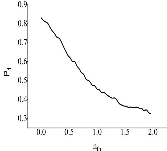
FIG. 3. The maximal values of population  $P_1(t)$  versus  $n_{th}$ . The parameters are:  $\Delta = 0$ ,  $\chi/\gamma = 15$ , the maximum amplitude of pump field  $\Omega/\gamma = 6$ ,  $\tau = 5.5\gamma^{-1}$ ,  $T = 0.4\gamma^{-1}$ .
