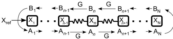
Figure 2: Scheme of a multi-agent system with a path-graph topology. The squares are agents with local dynamics described by (3) and (5). The virtual connections between the agents, which are created by the local control law, are illustrated by springs. All agents are identical.
