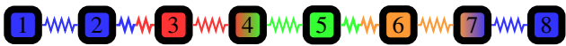
Figure 7: Schematic of the simulation setup for N = 8 . There are two soft boundaries (between 2, 3 and between 5, 6) and two hard boundaries (at agents 4, 7). Blue color corresponds to M_1 , red to M_2 , green to M_3 and orange to M_4 .
