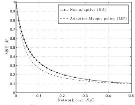
Figure 2. Trade-off between network cost and MSE.  $\alpha = 0.95$ ,  $c_{\text{TX}} = 1$ .
