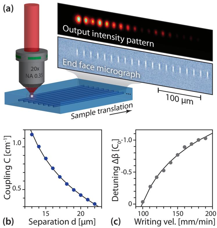
Fig. 2. (Color online) (a) Schematic of the waveguide inscription method. The inserts show a micrograph of the sample end face, and a typical output intensity pattern observed at 633 nm. (b) Dependence of the coupling coefficient  $C$  on the waveguide separation  $d$ . (c) Influence of the writing velocity on the detuning  $\Delta\beta$  of a waveguide with respect to a reference guide inscribed at 100 mm/min.
