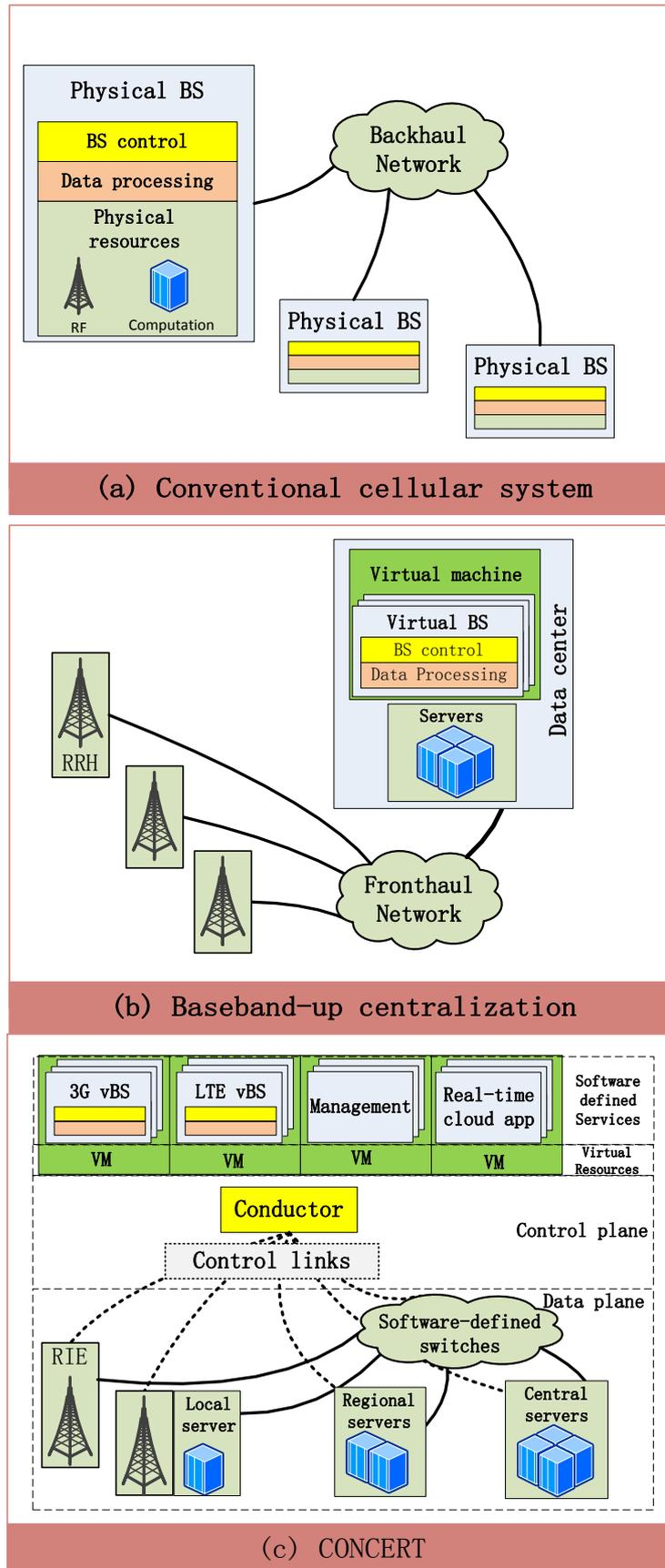
Figure 1 Comparison between conventional cellular systems, baseband-up centralization, and CONCERT architecture.
