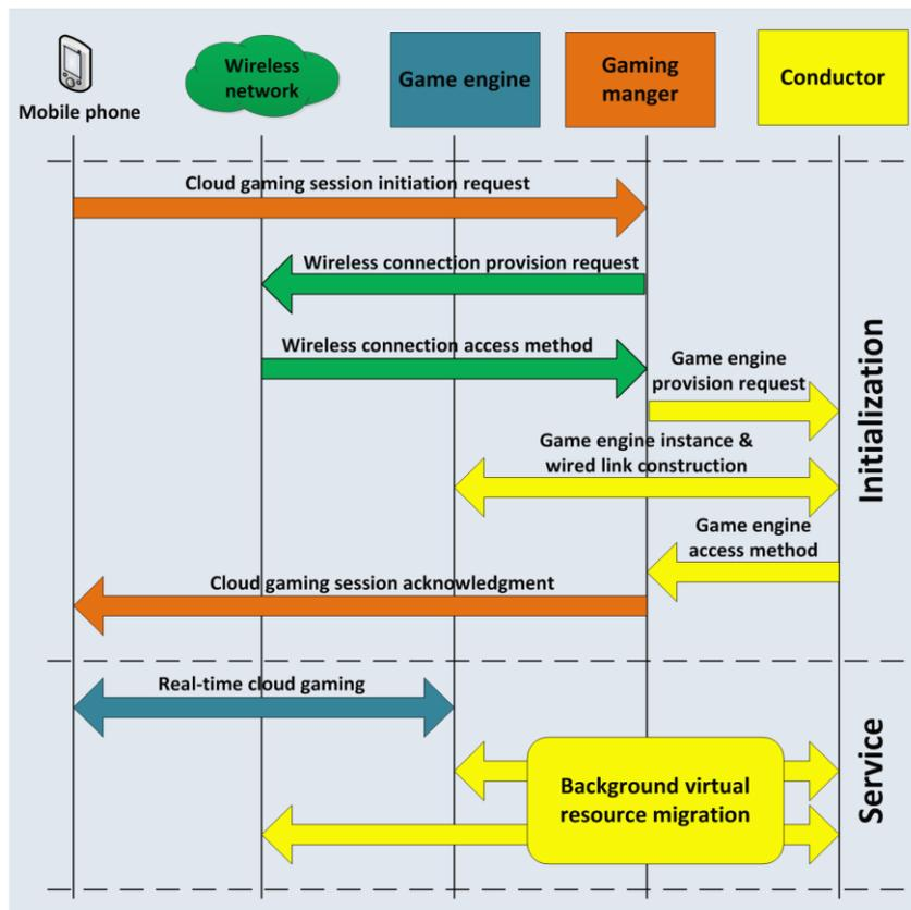
Figure 4 Signaling procedure of a cloud gaming service implemented in CONCERT
