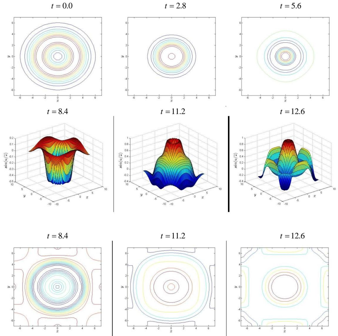
**Fig. 2.** Initial conditions and Numerical solutions of circular ring solitons at times  $t = 2.8, 5.6, 8.4, 11.2, 12.6$  with  $\Delta t = 0.2$ ,  $\Delta x = \Delta y = 0.4$ .
