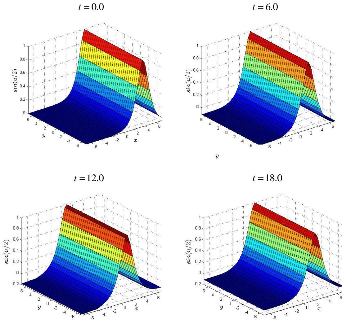
**Fig. 6.** Initial conditions and Numerical solutions of line soliton in an inhomogeneous medium at times  $t = 6.0, 12.0, 18.0$  with  $\Delta t = 0.001$  and grid size  $31 \times 31$ .
