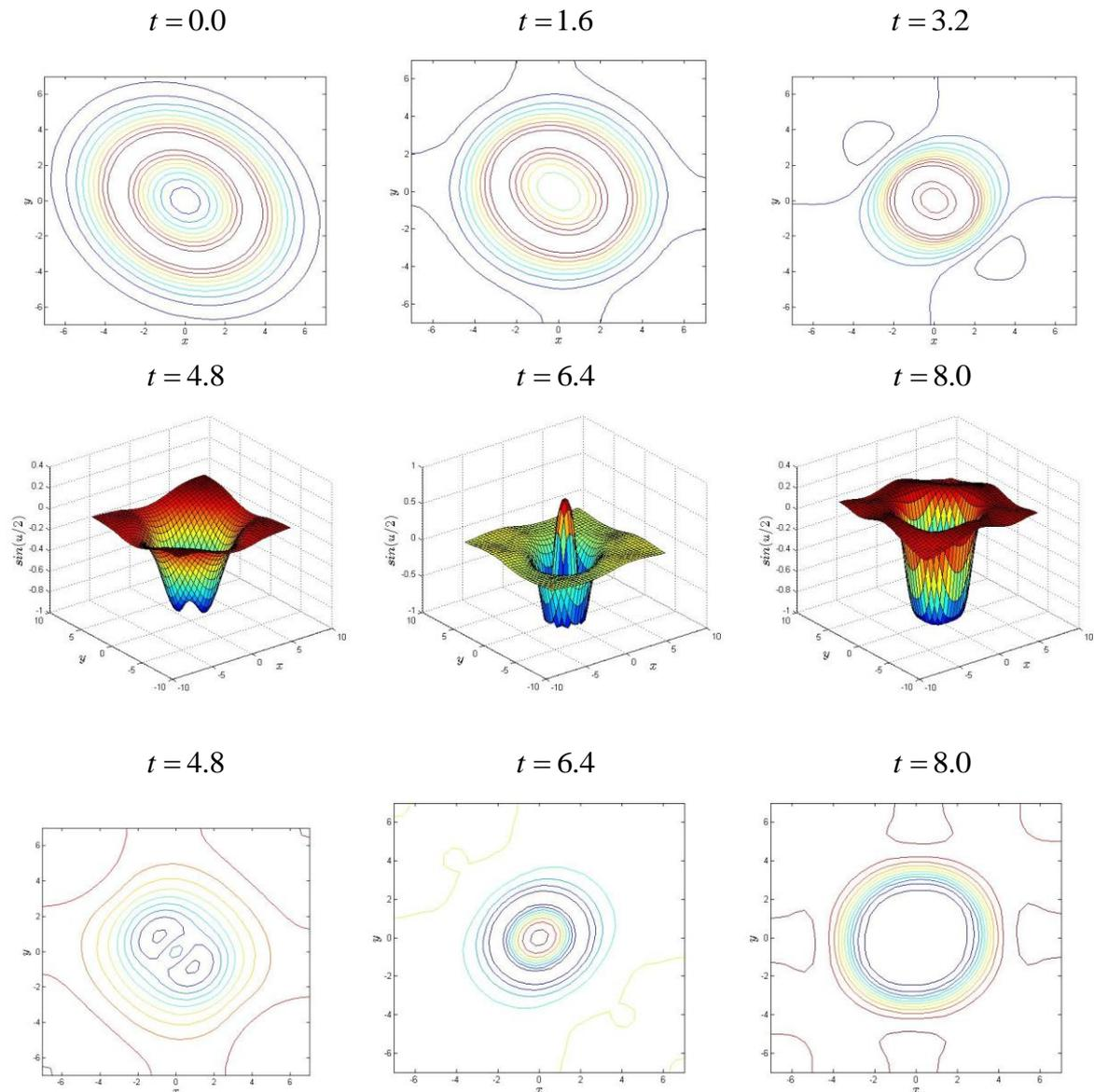
**Fig. 3.** Initial conditions and Numerical solutions of elliptical ring soliton at times  $t = 1.6, 3.2, 4.8, 6.4, 8.0, 9.6, 11.2$  with  $\Delta t = 0.2$ ,  $\Delta x = \Delta y = 0.4$ .
