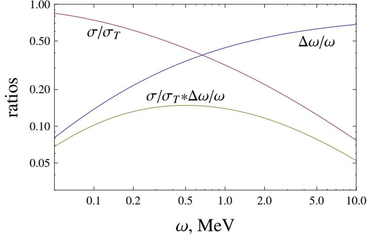
Figure 1: The ratio  $s = \sigma/\sigma_T$ , the mean relative energy transfer  $q = \Delta\omega/\omega$  and their product  $s \cdot q$  for Compton process is shown depending on photon energy.
