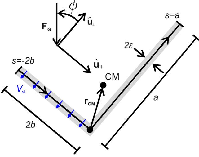
**Figure 5 | Sketch for the slender-body model.** Illustration of a rigid L-shaped particle with arm lengths  $a$  and  $2b$ . The position  $\mathbf{r}(t)$  of the center of mass CM and the orientation angle  $\phi(t)$  evolve over time due to the gravitational force  $\mathbf{F}_G$  and fluid slip velocity  $V_{sl}$  on the particle surface. The unit vectors  $\hat{\mathbf{u}}_{\parallel}$  and  $\hat{\mathbf{u}}_{\perp}$  indicate the particle-fixed coordinate system.
