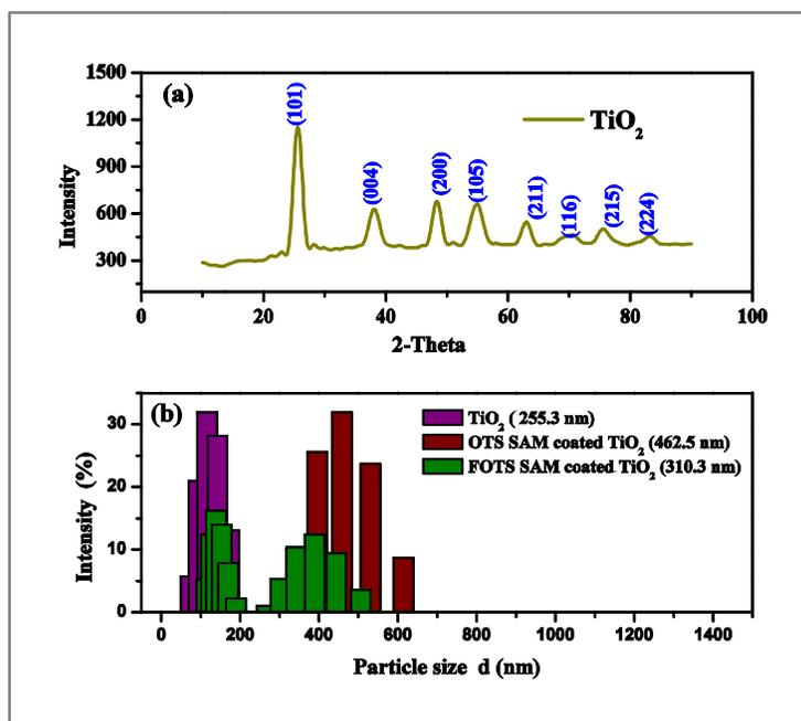
Fig.3. Shows (a) XRD spectrum of TiO<sub>2</sub> nanoparticles (b) The particle size distribution of uncoated, FOTS SAM and OTS SAM coated TiO<sub>2</sub> nanoparticles.
