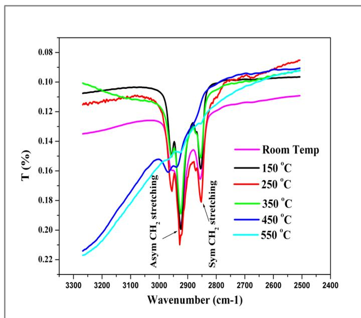
Fig.7. Shows symmetric and asymmetric stretching vibrations of  $\text{CH}_2$  functional groups.
