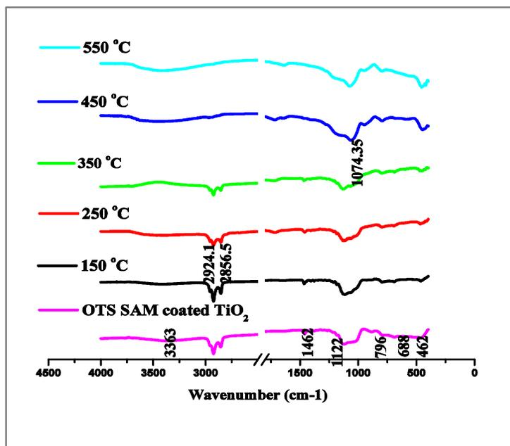
Fig.6. FTIR spectra of show thermal behavior for OTS SAM coated TiO<sub>2</sub> nanoparticles heat treated from room temperature to 550°C.
