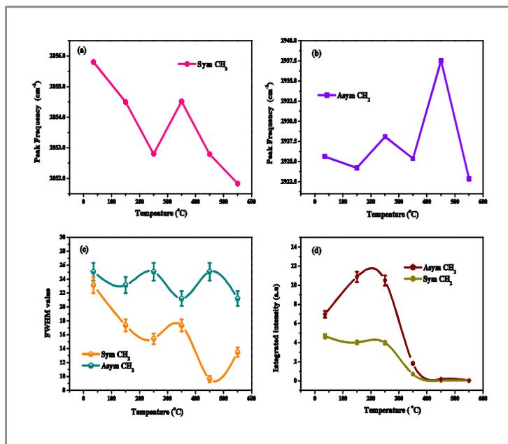
Fig.9. Shows thermal behavior of CH<sub>2</sub> symmetric and asymmetric vibrations (a) & (b) the peak frequency (c) FWHM and (d) Integrated Intensity.
