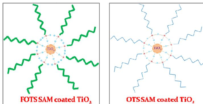
Fig.1. Shows (a) schematic diagram of FOTS SAM coated TiO<sub>2</sub> nanoparticle and (b) OTS SAM coated TiO<sub>2</sub> nanoparticle.
