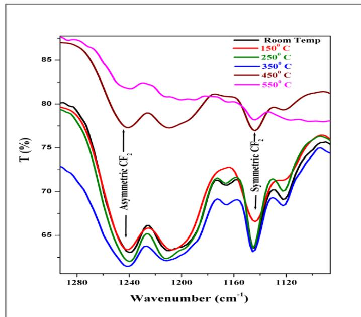
Fig.5. Shows symmetric and asymmetric stretching vibrations of CF<sub>2</sub> functional groups.
