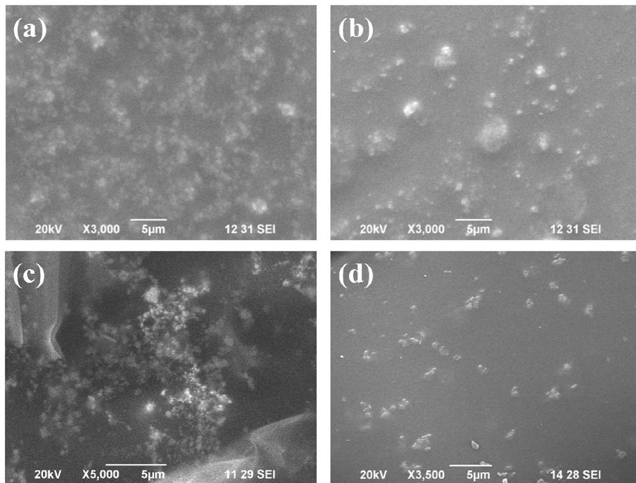
Fig.2. The nano-microstructure (a) and (b) FOTS SAM coated TiO<sub>2</sub> nanoparticles heat treated to 150°C and 450°C; (c) and (d) OTS SAM coated TiO<sub>2</sub> nanoparticles heat treated to 150°C and 450°C.
