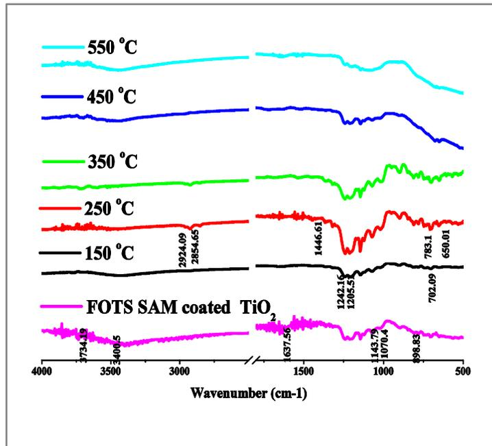
Fig.4. FTIR spectra show the thermal behavior of FOTS SAM coated TiO<sub>2</sub> nanoparticles heat treated from room temperature to 550°C.
