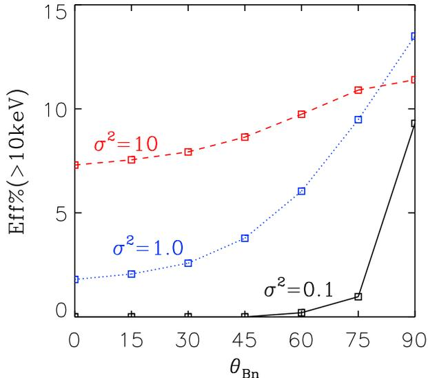
FIG. 2.— The efficiency of electron acceleration for various wave variances as a function of shock angle.  $\Gamma\%$  is defined by the fraction of electrons that is accelerated to more than 10 keV at the end of the simulations.
