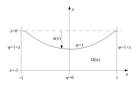
FIGURE 1. Idealized electrostatic MEMS device.
