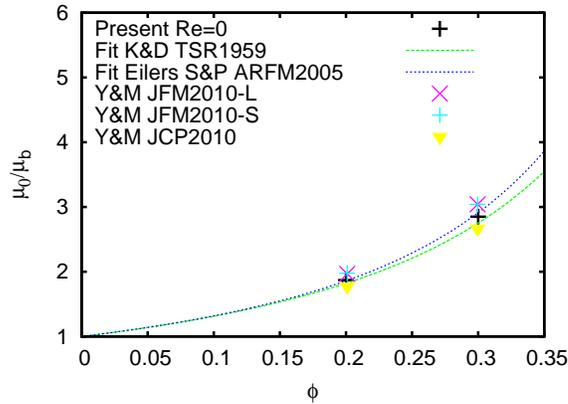
FIGURE 1. Relative viscosity  $\nu_r$  versus the volume fraction  $\Phi$  in a Couette flow in absence of inertia,  $Re = 0$ . The present data are compared with the results by Yeo & Maxey (2010*a,b*) and the Eilers Fit ( $1 + 1.25\Phi/(1 - \Phi/0.65)$ ).
