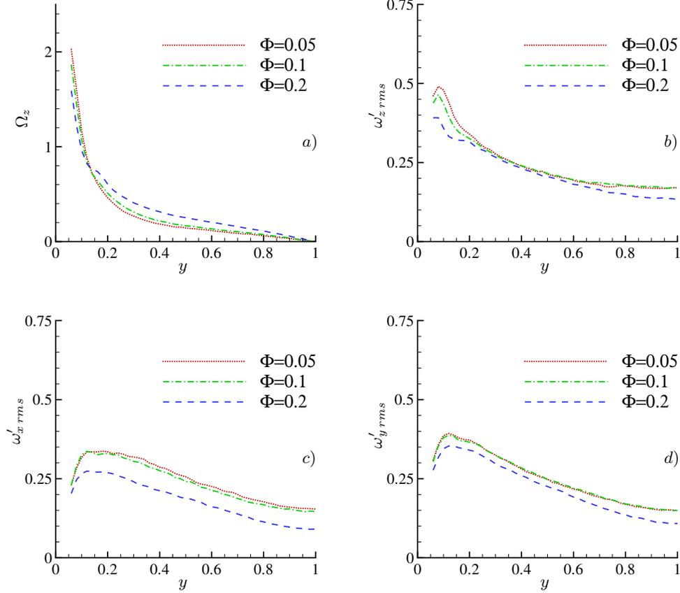
FIGURE 8. Particle angular velocity statistics in outer units for the different volume fractions  $\Phi$  studied. *a)* mean angular velocity (spanwise component)  $\Omega_z$ ; *b)* fluctuation rms of the spanwise fluctuation component  $\omega'_{z,rms}$ ; *c)* fluctuation rms of the streamwise component  $\omega'_{x,rms}$ ; *d)* fluctuation rms of the wall-normal component  $\omega'_{y,rms}$ .
