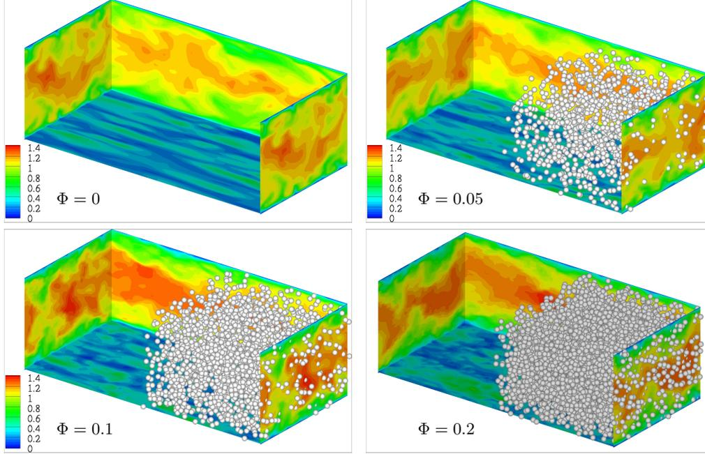
FIGURE 2. Instantaneous snapshots of the streamwise velocity on different orthogonal planes together with the corresponding particle position represented only on one half of the domain. The four panels represent the different values of the volume fraction under investigation,  $\Phi=0, 0.05, 0.1, 0.2$ .
