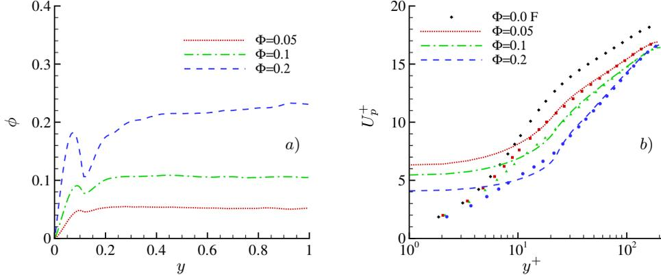
FIGURE 6. Particle average data for different nominal volume fractions  $\Phi$ . *a*) mean local volume fraction  $\phi$  versus the wall-normal coordinate  $y$  (maximum statistical error  $\pm 0.01$ ); *b*) mean particle velocity profile,  $U_p^+ = U_p/U_*$  in viscous units  $y^+ = y/\delta_*$  (lines) (maximum statistical error  $\pm 0.25 U_*$ ). The mean fluid velocity  $U_f^+$  is also reported for comparison (symbols).
