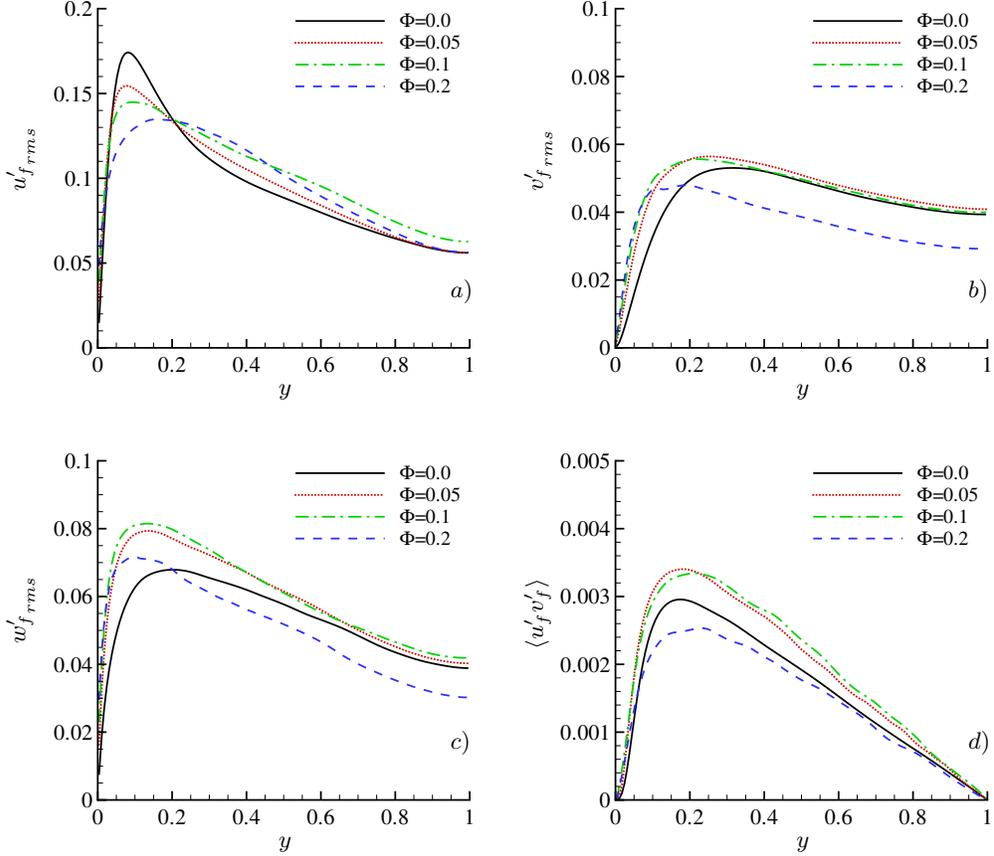
FIGURE 4. Intensity of the fluctuation velocity components and the Reynolds shear stress for the fluid phase in outer units for different volume fraction  $\Phi$ . Panel a) streamwise  $u'_{f,rms}$ ; b) wall-normal  $v'_{f,rms}$ ; c) spanwise  $w'_{f,rms}$  velocity fluctuations; d) shear-stress  $\langle u'_f v'_f \rangle$ .
