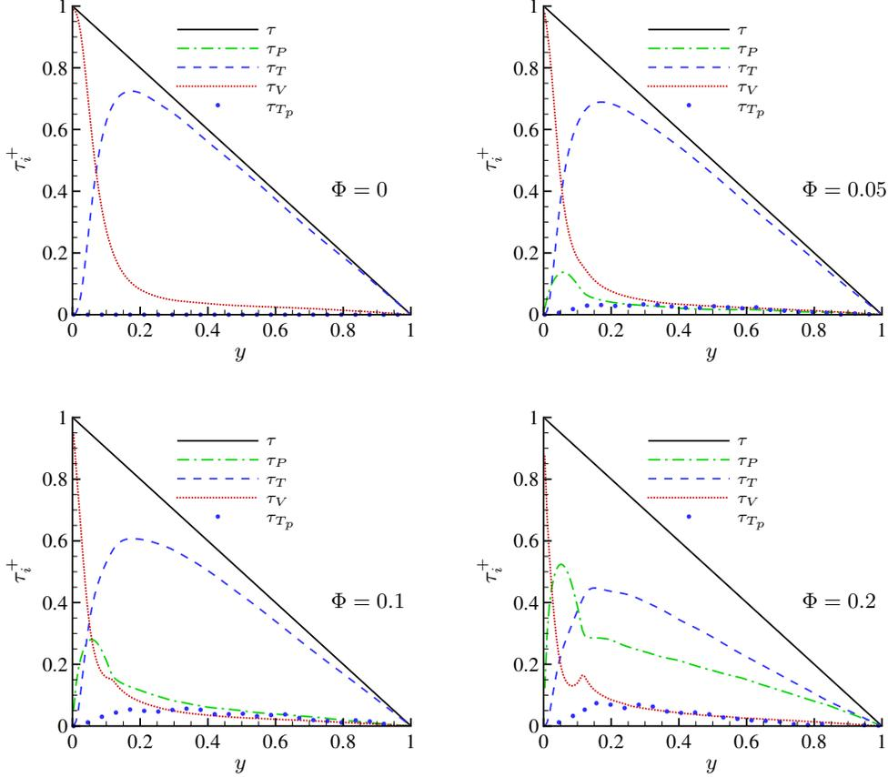
FIGURE 9. Momentum budget for the different bulk volume fractions  $\Phi$  under investigation. The wall is at  $y = 0$ , whereas  $y = 1$  is the channel centreline.  $\tau_V$ ,  $\tau_T$  and  $\tau_P$  represent the viscous, turbulent and particle induced stresses.  $\tau_{T_p}$  is the particle Reynolds stress and  $\tau = U_*^2 (1 - y)$  the total stress.
