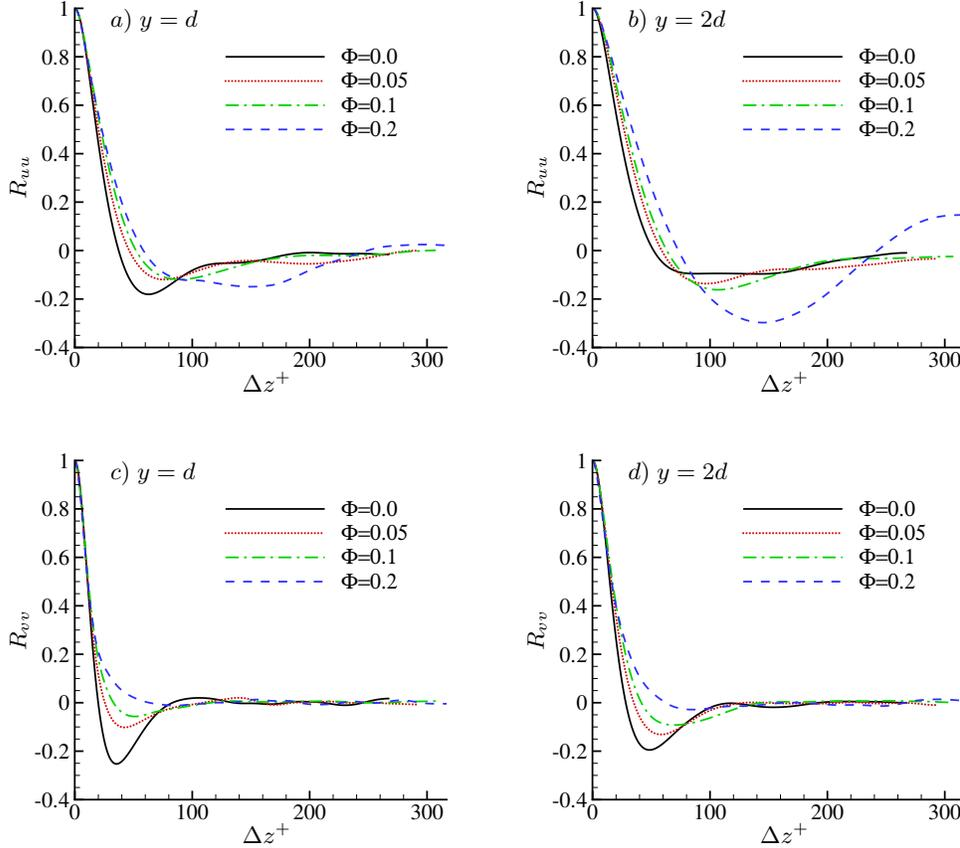
FIGURE 11. Correlations of the velocity fluctuations versus the spanwise separation  $\Delta z^+$  for different bulk volume fractions  $\Phi$ . Streamwise-streamwise component  $R_{uu}$  at a)  $y = d = h/18 \simeq 20\delta_*$  and b) at  $y = 2d = h/9 \simeq 40\delta_*$ . Wall-normal component  $R_{vv}$  at c)  $y = d = h/18 \simeq 20\delta_*$ , and d) at  $y = 2d = h/9 \simeq 40\delta_*$ .
