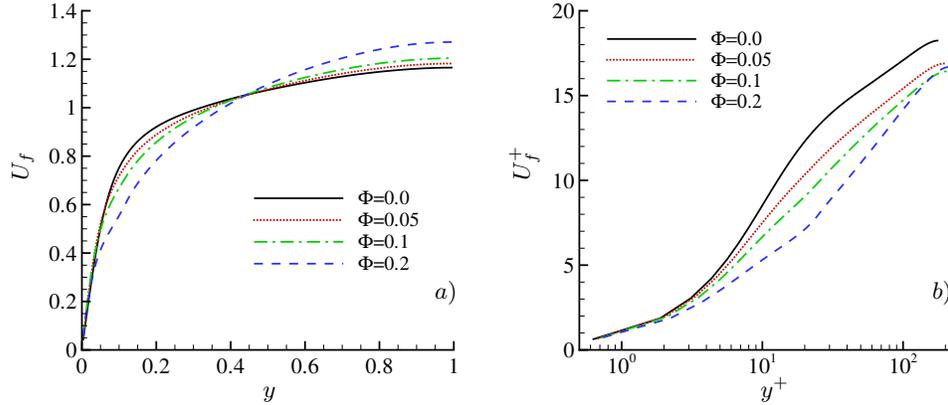
FIGURE 3. Mean fluid velocity profiles for the different volume fractions under investigations in a) outer units (hereafter wall normal distances without the superscript  $^+$  are assumed to be rescaled by  $h$ ) and b) inner units:  $U_f^+ = U_f/U_*$  vs  $y^+ = y/\delta_*$ , with  $U_*$  and  $\delta_*$  the friction velocity and viscous length scale, see definition in the text.
