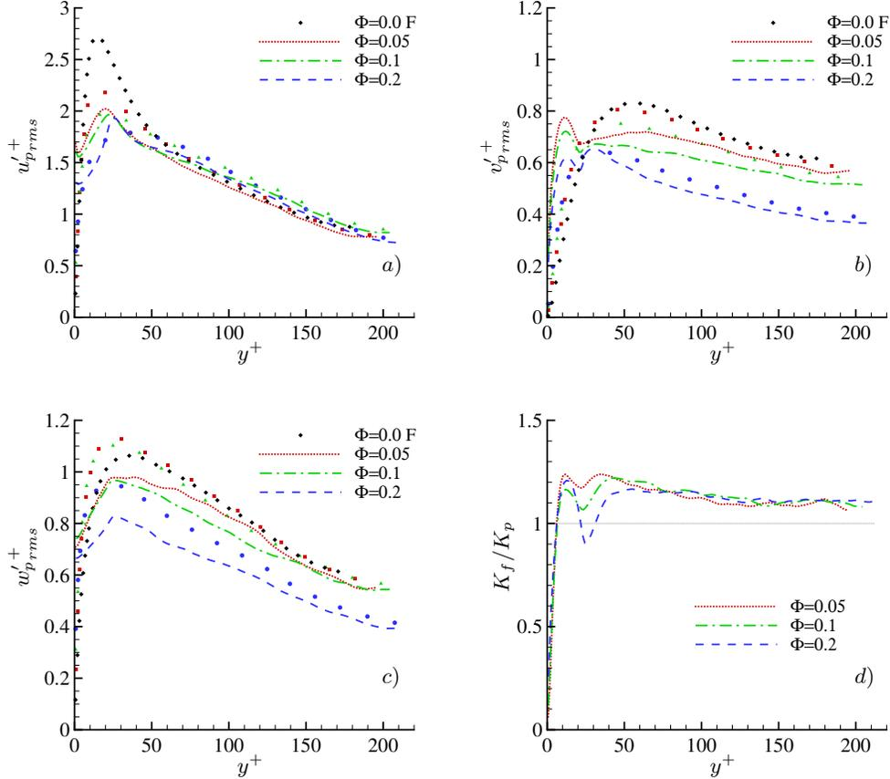
FIGURE 7. Intensity of the fluctuation velocity components for the solid phase in inner units for the different volume fraction  $\Phi$  studied (maximum statistical error  $\pm 0.06 U_*$ ). *a*) streamwise  $u'_{prms}+$ ; *b*) wall-normal  $v'_{prms}+$ ; and *c*) spanwise  $w'_{prms}+$  component. Symbols represent the fluctuation levels of the fluid phase. Panel *d*) displays the wall-normal profile of the ratio between the turbulent kinetic energy of the fluid and of the solid phase.
