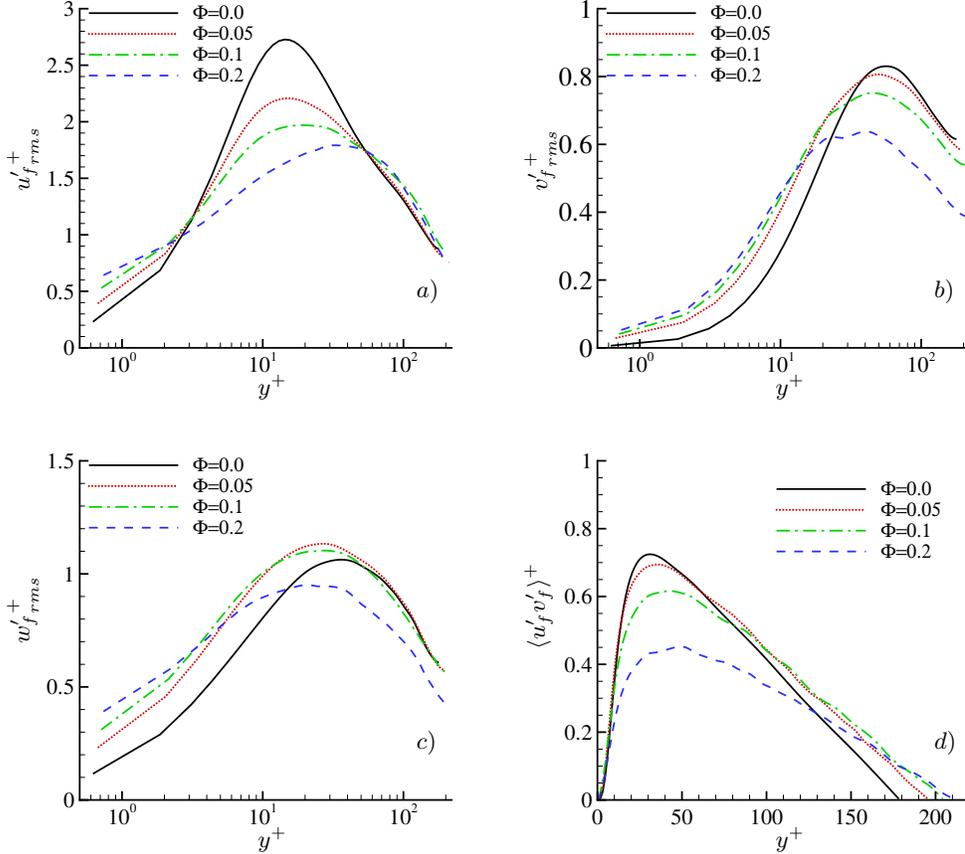
FIGURE 5. Intensity of the fluctuation velocity components and Reynolds shear stress for the fluid phase in inner units for different volume fraction  $\Phi$ . Panel a) streamwise  $u'_{f,rms}^+$ ; b) wall-normal  $v'_{f,rms}^+$ ; and c) spanwise  $w'_{f,rms}^+$  velocity component; d) shear-stress  $\langle u'_f v'_f \rangle^+$ .
