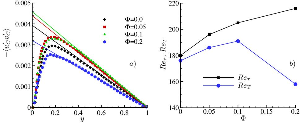
FIGURE 10. a): wall-normal profiles of the shear stress of the combined phase  $\langle u'_C v'_C \rangle / U_0^2$  (symbols) and linear fitting of the slope of the profile at the centreline,  $y = 1$ , depicted with solid lines. b): Friction Reynolds number  $Re_\tau = u_* h / \nu$  and Turbulent Friction Reynolds number  $Re_T = U_*^T h / \nu$  versus the bulk volume fraction  $\Phi$  from the simulations presented here.
