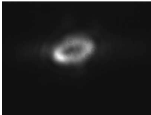
Figure 8: Beam image at 1.4 GeV after the third chicane at SACLA showing the COTR halo in the near field [11].
