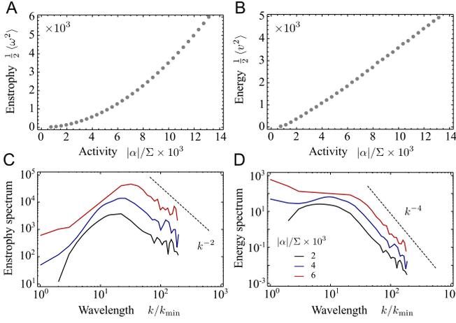
FIG. 5: Enstrophy (A) and energy (B) per unit area versus activity. The data show, respectively, quadratic and linear scaling. (C) Enstrophy and (D) energy spectra for three activity values. The wavelength is normalized to unity at  $k_{\min} = 2\pi/L$ .
