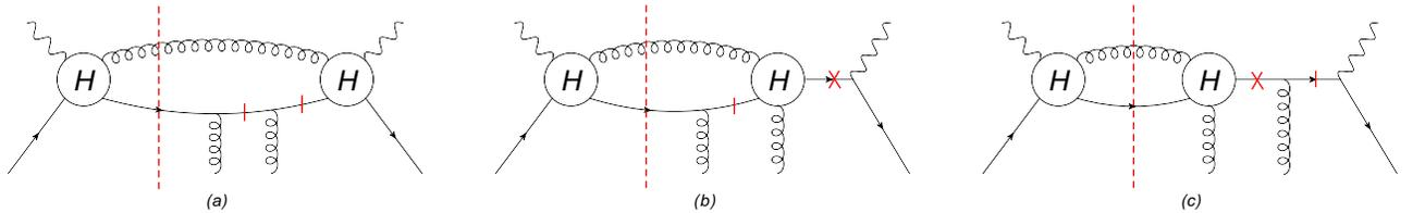
FIG. 7. The left-cut diagrams for (a) soft-soft, (b) soft-hard, and (c) hard-soft rescattering processes in SIDIS. The short bars (crosses) indicate the propagators where the soft (hard) poles arise.
