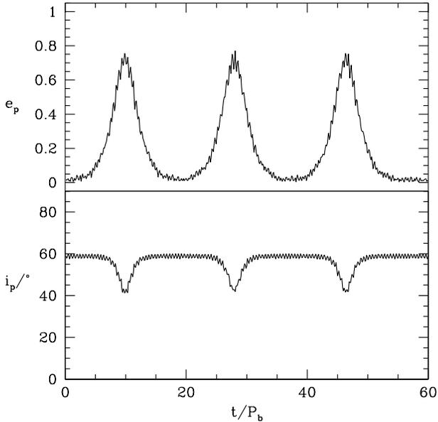
FIG. 1.— The eccentricity and inclination evolution of a test particle around the primary of an equal mass binary. The particle is initially at a radius  $d = 0.2a$  in a circular orbit from the primary mass at an inclination  $i_{p0} = 60^\circ$ .
