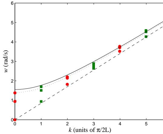
FIG. 9. Dependence of the dispersion on gravity in the long-rod wave machine in the low- $k$  region. The solid curve corresponds to one  $g$ , the dotted curve corresponds to one-half  $g$ , and the dashed line corresponds to zero- $g$ .
