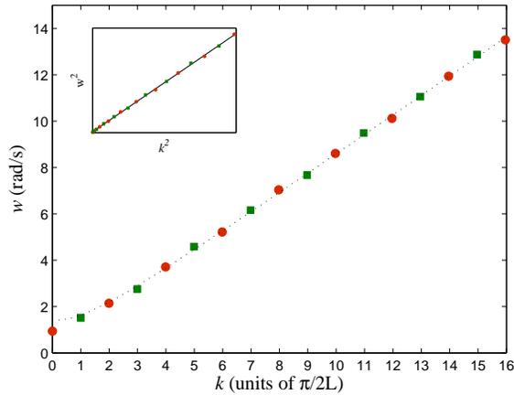
FIG. 7. Harmonics of the long-rod wave machine in a half- $g$  environment, and comparison with the dispersion relation given by Eq. (8) (dotted curve). The red circles represent the free-end harmonics, and the green squares represent the fixed-end harmonics. The inset displays the linear regression of the  $\omega^2$  vs.  $k^2$  data points.
