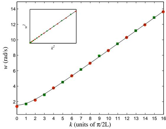
FIG. 6. Harmonics of the long-rod wave machine in a one- $g$  environment, and comparison with the dispersion relation given by Eq. (8) (solid curve). The red circles represent the free-end harmonics and the green squares represent the fixed-end harmonics. The inset displays the linear regression of the  $\omega^2$  vs.  $k^2$  data points.
