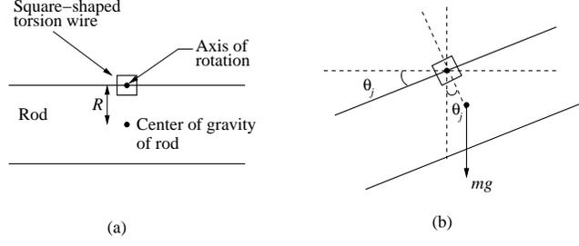
FIG. 2. Rod in (a) equilibrium position, and (b) tilted by an angle  $\theta_j$ . Because the center-of-gravity of the rod is below the axis of rotation, the weight  $mg$  of the rod produces a restoring gravitational torque of magnitude  $mgR \sin(\theta_j)$ .
