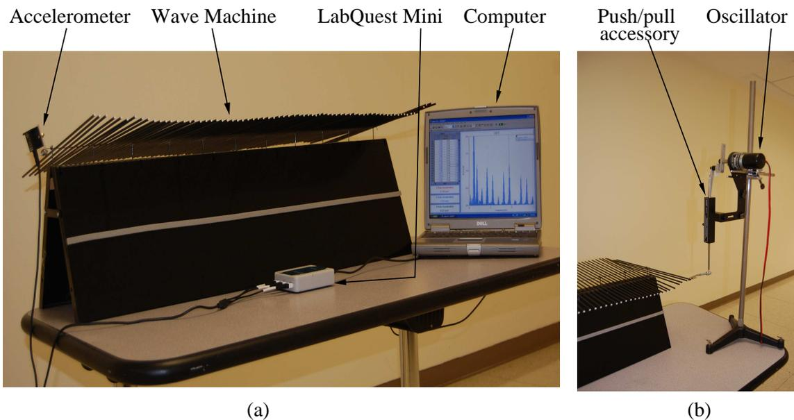
FIG. 1. (a) Experimental apparatus. (b) The oscillator drives the wave machine through PASCO's push/pull accessory, which is attached to one of the end rods.
