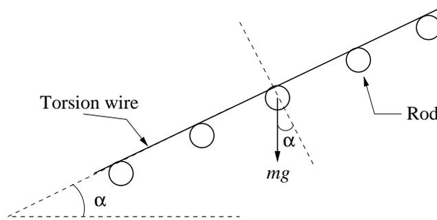
FIG. 5. Wave machine tilted by an angle  $\alpha$ . The component of each rod's weight parallel to the torsion wire ( $mg \sin \alpha$ ) does not produce any torque. Only the component of the rod's weight perpendicular to the torsion wire ( $mg \cos \alpha$ ) produces a torque. Hence, tilting the wave machine by an angle  $\alpha$  effectively reduces the strength of gravity to  $g \cos \alpha$ .
