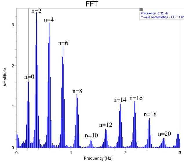
FIG. 4. FFT frequency spectrum of a wave pulse sent through the long-rod wave machine in a one- $g$  environment with free ends. By clicking on the center of each peak, the harmonic frequency is displayed in an inset at the top right corner. The pendulum mode ( $n = 0$ ) corresponds to the peak of lowest frequency (0.22 Hz).
