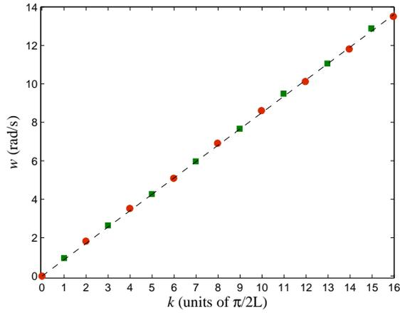
FIG. 8. Harmonics of the long-rod wave machine in a zero- $g$  environment, and comparison with the dispersion relation given by Eq. (12) (dashed line). The red circles represent the free-end harmonics, and the green squares represent the fixed-end harmonics.
