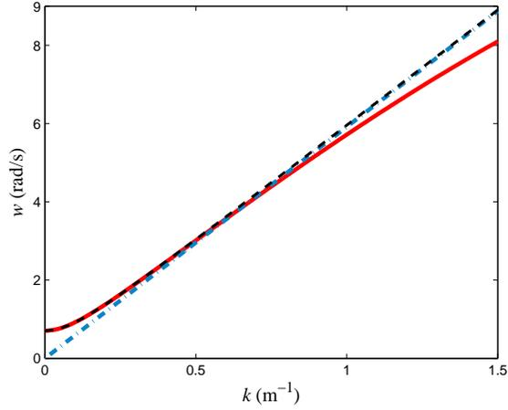
FIG. 3. Plots of the dispersion relations: Eq. (5) (red, solid line), Eq. (8) (black, vertically-dashed line), and Eq. (12) (blue, dash-dot line). The plots correspond to  $c = \sqrt{35}$  m/s,  $\omega_p = 0.5$  rad/s,  $\omega_t = 1$  rad/s, and  $d = 1$  m.
