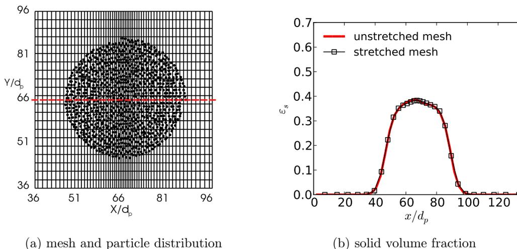
Figure 13: Comparison between solid volume fraction obtained with uniform mesh and stretched mesh using diffusion-based averaging method. Panel (a) displays the mesh and the particle distribution in the shaded region in Fig. 7(a). The mesh is stretched in  $x$ -direction with a resolution of  $N_x \times N_y = 90 \times 45$ . Panel (b) shows the solid volume fraction along the horizontal centerline of the domain (dashed line in panel (a)).
