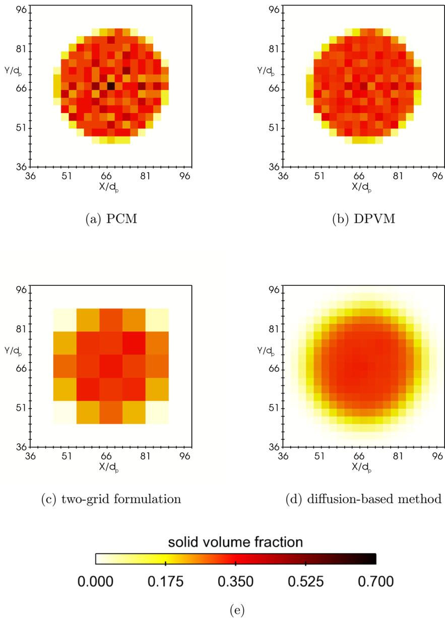
Figure 12: Comparison of the solid volume fraction  $\varepsilon_s$  fields obtained by using the four coarse graining method: (a) PCM, (b) DPVM, (c) the two-grid formulation, and (d) the diffusion-based method. The particle distribution and the meshes used to obtain the plots for PCM, DPVM, and the diffusion-based method are shown in Fig. 8(a) and those for the two-grid formulation are shown in Fig. 11(a).
