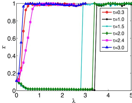
FIG. 2. (Color online) The order parameter  $r$  as a function of coupling strength  $\lambda$  with different values of time-delay  $\tau$  introduced in a star network of  $K = 50$  leaves with  $m = 1$ . For different values of time delay, the star network represents different synchronization transition.
