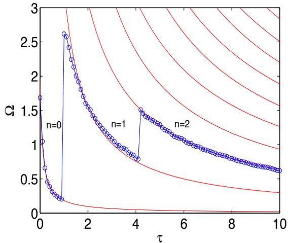
FIG. 3. (Color online) The average frequency  $\Omega$  (or  $C$ ) as a function of the time delay  $\tau$  for the coupling strength  $\lambda = 5$  in a star network of  $K = 50$  leaves. The circles  $\circ$  represent the simulation result, and solid lines represent the theoretical prediction by Eq.(9) while considering  $\Omega\tau \rightarrow (\Omega\tau - n\pi)$ . There is an oscillatory dependence of  $\Omega$  on the time delay  $\tau$ .
