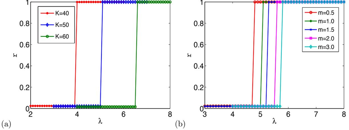
FIG. 1. (Color online) (a) Synchronization diagram ( $r - \lambda$ ) for the star networks of different sizes  $K = 40, 50$  and  $60$  corresponding to  $m = 1$ . First order transition is observed in the star network when degree - frequency correlation is taken into account. (b) Synchronization diagram ( $r - \lambda$ ) for a star network of  $K = 50$  leaves for different values of  $m$ .
