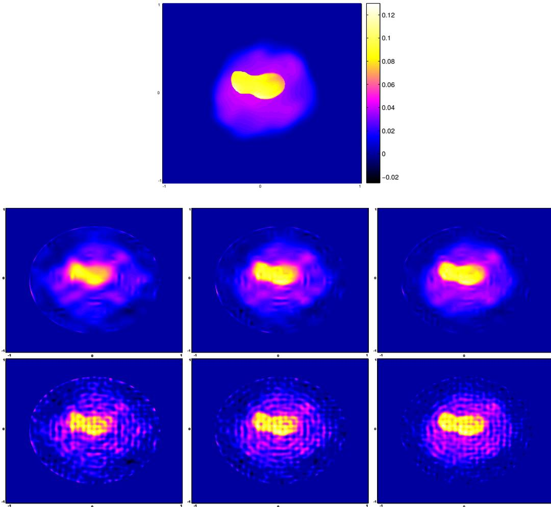
Figure 3: **Top:** Scatterer. **Second Row:** Reconstructed scatterers using the shearlet regularization, noise levels from left to right:  $\varepsilon = 0.005, 0.002, 0.001$ . **Third Row:** Reconstructed scatterers using the  $L^1$  regularization, noise levels from left to right:  $\varepsilon = 0.005, 0.002, 0.001$ .
