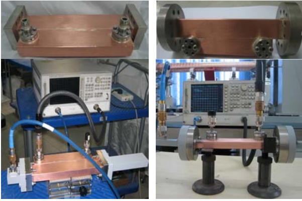
(a) C-band coupler (b) X-band coupler Fig. 4 Prototype and testing of the waveguide directional couplers
