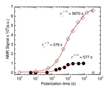
FIG. 2. Build-up on the nuclear spin polarization by 1047 nm laser irradiation for up to ~10 h, at 1.7 K and 4.2 K temperature respectively. The red lines represent a bi-exponential fit with time constants,  $\tau_1 = 5670$  s and  $\tau_2 = 578$  s at 1.7 K, and an exponential fit with  $\tau = 577$  s at 4.2 K. The star represents a thermal polarization measurement (laser off) for ~10 h, at 1.7 K, where no polarization could be observed.
