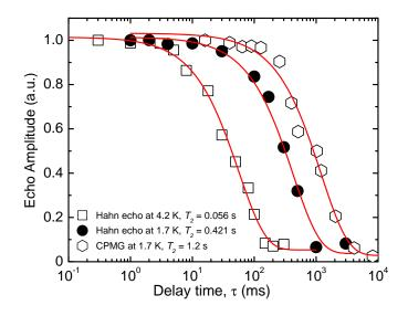
FIG. 3. Nuclear spin coherence time,  $T_2$ , measured with the Hahn echo at 4.2 K temperature, open squares, Hahn echo at 1.7 K, full circles, and CPMG pulse sequence at 1.7 K, open diamonds. All data were measured in 6.7 T field, with 200 s of optical polarization provided by a 1047 nm, 100 mW, above-gap laser.
