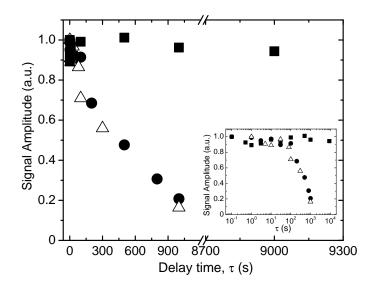
FIG. 4. Nuclear spin relaxation time,  $T_1$ , measured with a simple  $\pi/2$  read-out pulse at 4.2 K (open triangles) and 1.7 K (black squares), respectively, and with an inversion recovery pulse sequence (closed circles) at 4.2 K.
