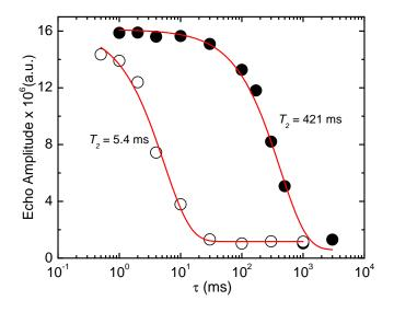
FIG. 5. Nuclear spin coherence time,  $T_2$ , measured with the Hahn echo at 1.7 K temperature in 6.7 T field. Closed symbols represent a situation where the laser is OFF during the acquisition. Open symbols show data taken using the same pulse sequence but keeping the laser ON during the acquisition.
