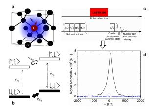
FIG. 1. Raw spectrum of <sup>31</sup>P-nuclear spins in <sup>28</sup>Si crystal, at 1.7 K in 6.7 T. The data were taken by applying only one  $\pi/2$  pulse and recording the FID. SNR is 113. a) Schematic and b) eletronic structure of the donor impurity. c) Pulse sequence used to obtain spectrum in d).
