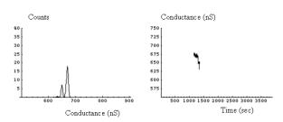
Fig. 7. Influenza + Parmyoxovirus histogram and data window containing possible virus sequential bind signature – local mean at a conductance of roughly 675 nS.
