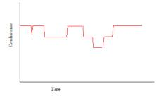
Fig. 1. Idealized conductance trace showing, respectively, nonspecific transient spike, specific binding, and superimposed specific bindings.
