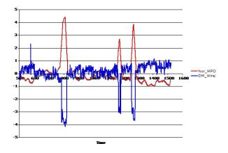
Fig. 4. Normalized conductance trace with matched filter output.
