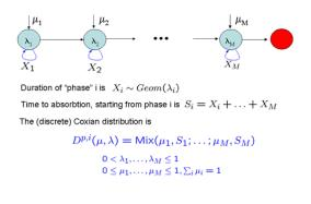
Fig. 17. Markov model representation of multiphase Coxian distribution [4].
