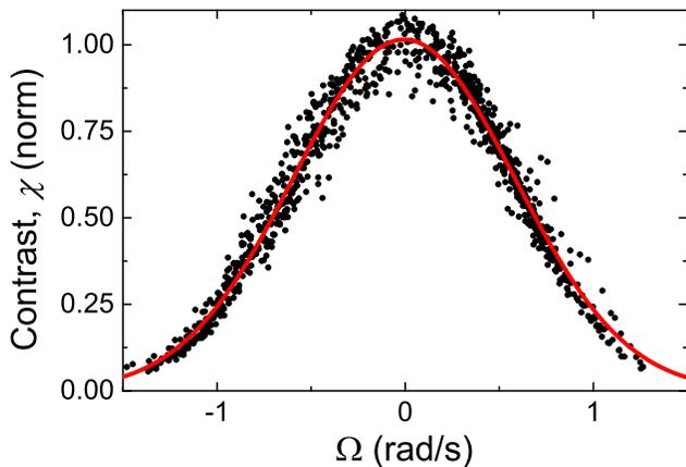
FIG. 8. (Color online) Contrast loss under high rotation rate. The black points are the observed fringe contrast as the apparatus was rotated in the  $\pm\hat{\mathbf{g}}$  direction, up to  $\pm 1.5$  rad/s. The red line is a Gaussian fit, with a width of  $\sigma = 0.60(1)$  rad/s.
