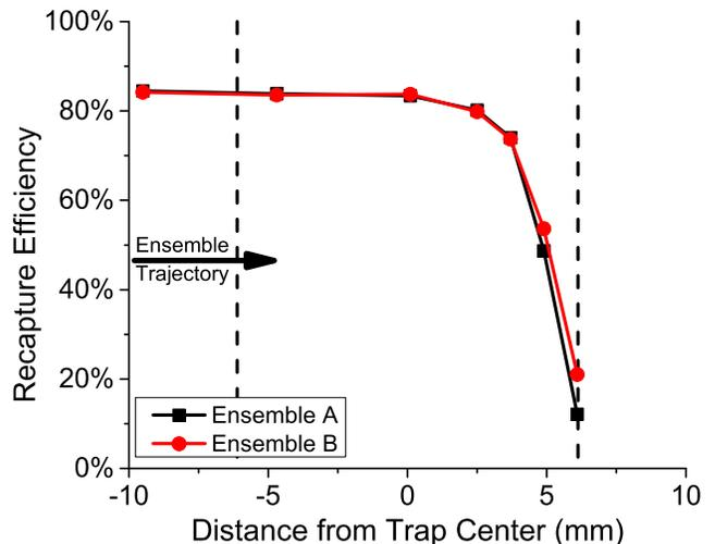
FIG. 7. (Color online) Recapture efficiency over a range of ensemble positions relative to the trap center, at the onset of ballistic recapture. Dashed lines represent the  $1/e^2$  diameter of the trapping volume. For early onset (negative position), the ensemble's momentum still carries it into the trap. Recapture is still efficient over a large fraction of the trap volume.
