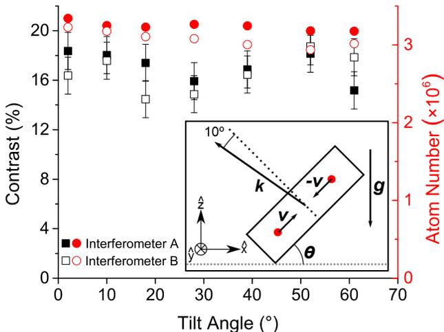
FIG. 6. (Color online) Immunity of the atom interferometer to a range of tilt. The tilt direction corresponds to  $\theta_y$ , thus changing the projection of gravity on the Raman beam axis, as well as the launch axis. Error bars represent the long-term drift seen in the apparatus over 1 hr when the interferometer is flat on the table. The fringe contrast and steady-state atom number are largely unaffected by the orientation.
