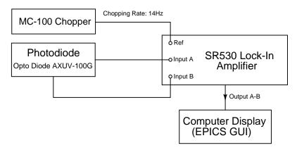
Figure 2. A schematic diagram of the signal input and output through the SR530 lock-in amplifier.
