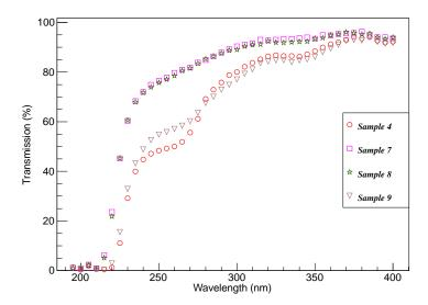
**Figure 8.** Heat study: Transmission curves for samples of similar thicknesses (masses) cured by different methods. Note that samples #7 and #8 measure 1.48 mm and 1.37 mm in thickness, where #7 was cured via the heat method. Samples #4 and #9 measure 3.35 mm and 3.39 mm in thickness, where #9 was cured with heat method. The standard deviations due to the six reference spectra are smaller than the plotting symbols.
