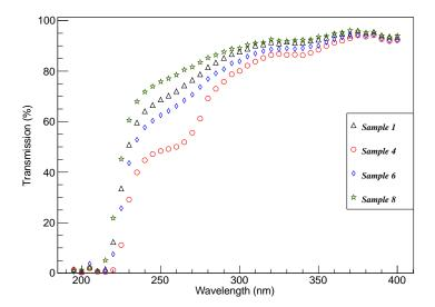
**Figure 4.** RTV thickness study: Transmission results for normal cured samples #1, #4, #6 and #8. Note that sample #8 has the smallest and #4 has the largest thickness. The errors in the transmissions, estimated from the standard deviation when applying the six reference spectra to each measurement spectrum, are smaller than the plotting symbols.
