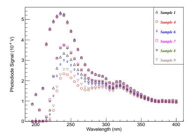
**Figure 3.** Response spectra as measured by a 1 cm  $\times$  1 cm UV sensitive photodiode [5]. The upper symbols are the reference spectra, and the lower symbols are the measurement spectra.
