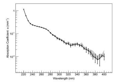
**Figure 7.** Final absorption coefficient ( $\alpha$ ) results for Momentive RTV615 with normal curing method. The description for the curves and errors are the same as Fig. 6. The total uncertainty in  $\alpha$  at any wavelength is the arithmetic sum of the error bar and shaded error band.
