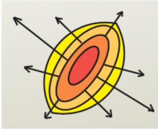
According to the laws of fluid mechanics, as we shall prove them, this implies that an acceleration field is generated from high pressures to low pressures.
