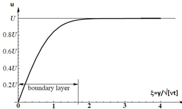
The region in which the velocity field departs significantly from the constant flow  $U$  is called boundary layer: according to the expression of  $u(y, t)$ , this layer is proportional to  $\sqrt{vt}$ . Hence, for fixed time, the boundary layer decreases as  $1/\sqrt{\operatorname{Re}}$ .
