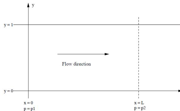
We are looking for a stationary solution of Navier-Stokes equations of the form  $\mathbf{v}=(u(x, y), 0)$ . Indeed, the flow is directed only along the  $x$ -axis. With:  $p=p(x)$  and  $p(0)=p_1$ ,  $p(L)=p_2$ . The continuity equation for incompressible fluid gives  $\partial_x u = 0$ , where we use the standard notation  $\partial_x = \partial / \partial x$ . Hence  $u(x,y)=u(y)$  and  $\mathbf{v}=(u(y), 0)$ . The Navier-Stokes equation for the only component to be considered reads:
