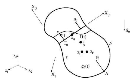
Figure 2. General view of the sloshing problem in a six degrees of freedom rigid body. The free boundary  $\Gamma(t)$  is issued from the equilibrium free boundary at rest  $\Gamma_0$  with the help of the elongation  $\eta$ . The other notations are explained in the corpus of the text.
