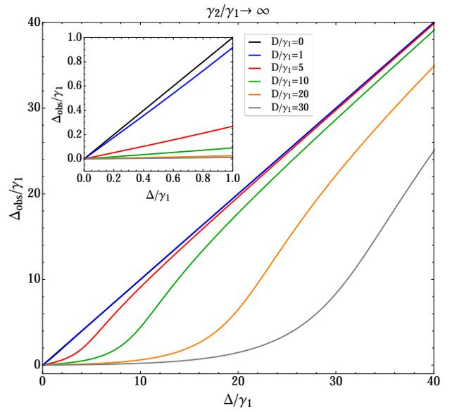
FIG. 3: Observed detuning  $\Delta_{\text{obs}} = |\tilde{\omega}_2 - \tilde{\omega}_1|$  as a function of the initial detuning  $\Delta = |\omega_2 - \omega_1|$  for various coupling strengths  $D$  and  $\gamma_2/\gamma_1 \rightarrow \infty$ . Increasing the coupling strength leads to frequency entrainment of the two quantum VdP oscillators. A well-defined synchronization plateau as one would expect for classical noiseless VdP oscillators is absent due to the unavoidable quantum noise.
