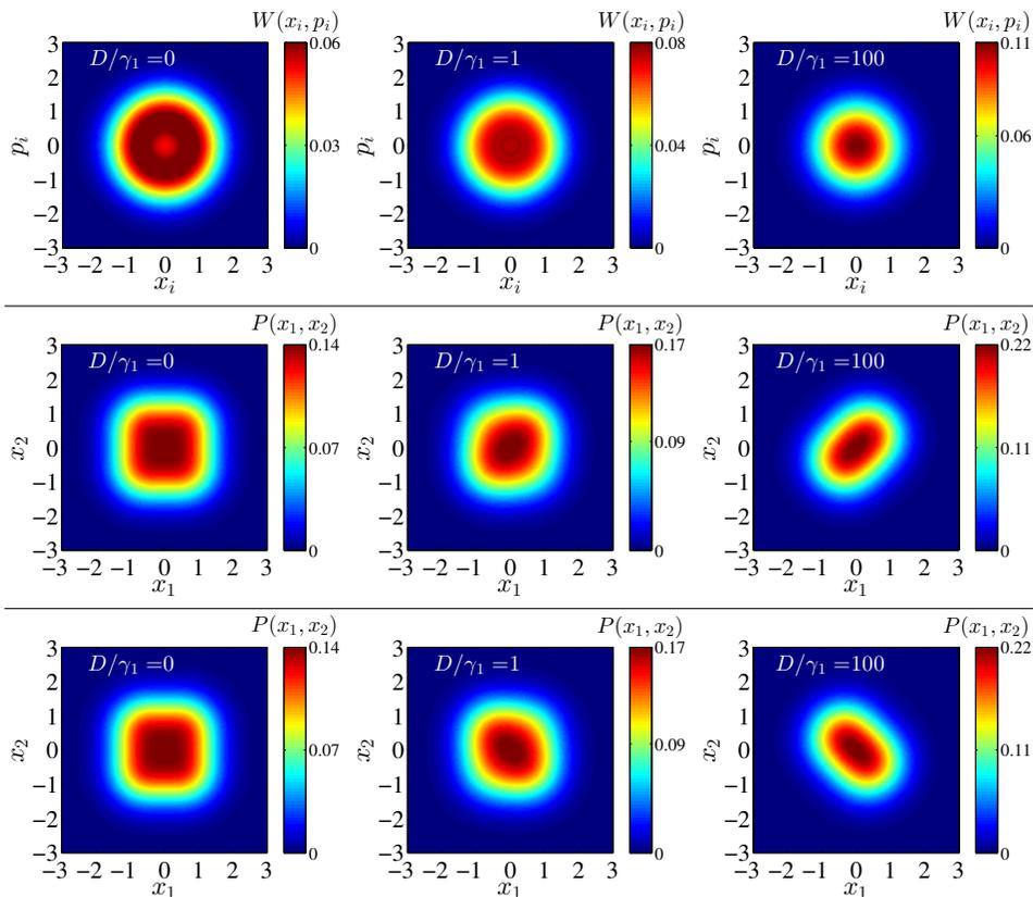
FIG. 1: Wigner function  $W(x_1, p_1) = W(x_2, p_2)$  (first row) and joint-probability distribution  $P(x_1, x_2)$  (second and third row) for different coupling strengths  $D$  increasing from left to right. In the second row we show the results for the dissipator  $\mathcal{D}[a_1 - a_2]$  and in the third row for  $\mathcal{D}[a_1 + a_2]$ . In all cases  $\gamma_2/\gamma_1 = 100$  and  $\Delta/\gamma_1 = 0.4$ .
