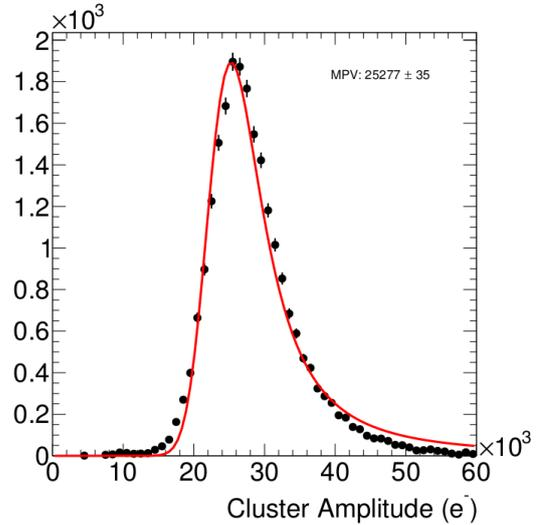
Figure 12: The cluster charge distribution for hits associated with a track follow the characteristic Landau shape.
