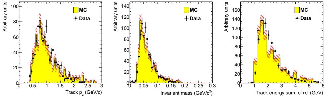
Figure 15: Kinematic distributions for  $e^+e^-$  pairs selected by opposite charged tracks in the top and bottom half of the tracker: track momentum in the top half of the SVT (left), invariant mass (middle) and the sum of the track energy for the pair (right).
