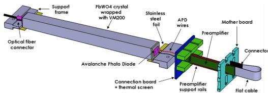
Figure 6: A schematic view of an ECal module.
