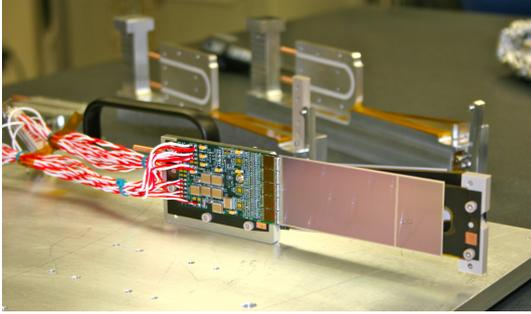
Figure 5: A prototype module assembly (foreground) with the 50 mrad (left) and 100 mrad (right) module assembly fixtures in the background. A pair of cooling blocks and a spacer block can be seen on the fixtures.
