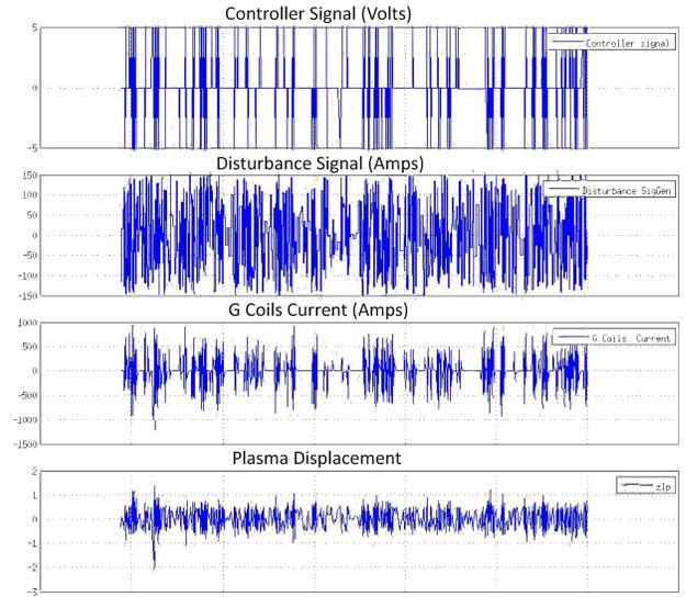
Fig. 5. Simulation results of the bang-bang controller.
