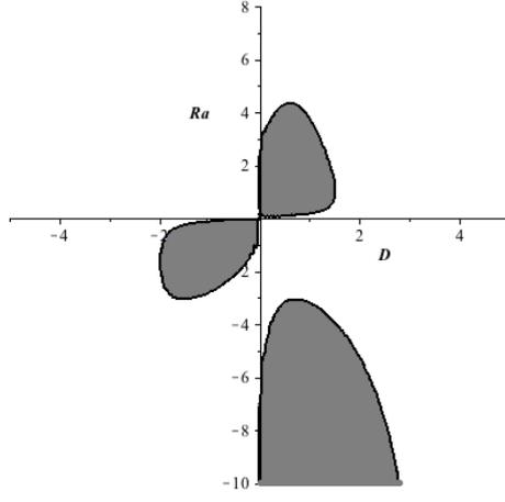
Figure 1: Instability condition with negative temperature gradient
