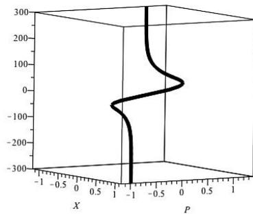
Figure 6: Helical Kinks between two nodes, with  $D = 1,5$ ,  $Ra = 1,9$ ,  $C_1 = 0,05$ ,  $C_2 = 0,01$ .
