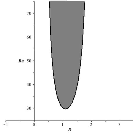
Figure 2: Instability condition with positive temperature gradient
