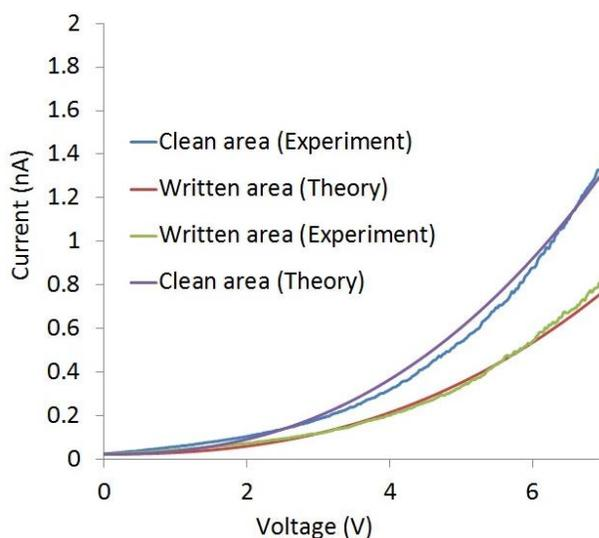
**Fig. 6: EGDM model.** Current-Voltage characteristic as for P3HT:[70]PCBM annealed at 100 °C (blend involving higher molecular weight P3HT) for unwritten region and written region in same experiment, recorded at room temperature ( $T=300\text{K}$ ) and comparison with EGDM model. In the clean area the width of the Gaussian DOS is  $\sigma=0.11\text{eV}$ , while  $\sigma=0.116\text{eV}$  in the written region. Experimental curves are average over 5 measurements.
