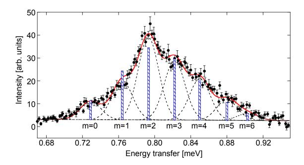
FIG. 2. (Color online) Energy distribution of the  $Mn^{2+}$  singlet-triplet dimer transition observed for  $KMn_{0.10}Zn_{0.90}F_3$  at T=2 K. The lines are the result of a least-squares fitting procedure as explained in the text. The vertical bars correspond to the probabilities  $p_m(x)$  predicted by Eq. (1) with n=26.
