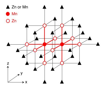
FIG. 3. (Color online) Three-dimensional sketch of the structure of  $KMn_xZn_{1-x}F_3$  (only the Mn and Zn positions are shown). The triangles denote the 26 nearest-neighbor positions around the central  $Mn^{2+}$  dimer marked by spheres.
