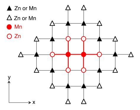
FIG. 5. (Color online) Two-dimensional sketch of the structure of  $K_2Mn_xZn_{1-x}F_4$  (only the Mn and Zn positions are shown). The full and open triangles denote the 10 nearest-neighbor and 14 next-nearest-neighbor positions, respectively, around the central  $Mn^{2+}$  dimer marked by spheres.
