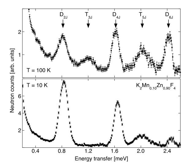
FIG. 1. Energy spectra of neutrons scattered from  $K_2Mn_{0.10}Zn_{0.90}F_4$ . The incoming neutron energy was 4.2 meV. The arrows mark the multimer transitions (D=dimer, T=trimer) with energies indicated by the subscript zJ.
