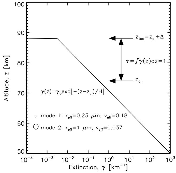
**Fig. B.3.** Sketch that illustrates the meaning of the parameters in our prescribed model atmosphere.
