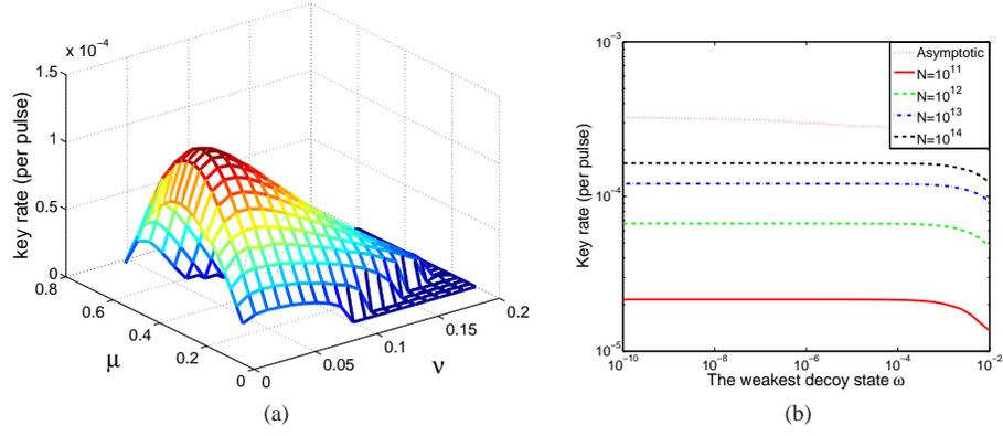
FIG. 7: (Color online) (a) Convexity of key rate function. The key rate is simulated by sweeping  $\mu$  and  $\nu$ , and optimizing other parameters. (b) Key rate as a function of the decoy state  $\omega$ . As long as the intensity of  $\omega$  is below  $1 \times 10^{-3}$ , the key rate is very close to the optimum. A perfect vacuum ( $\omega = 0$ ) is not essentially required in practical decoy-state QKD experiments.
