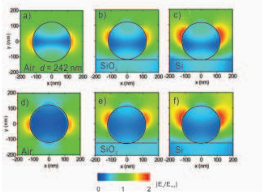
Figure 1. Screening of incident plane wave by InP NWs (diameter  $d = 242 \pm 7$  nm) inside the air and on different substrates with wavelengths  $\lambda = 1,200$  nm ((a), (b), and (c)) and  $\lambda = 1,500$  nm ((d), (e), and (f)). Figures are color maps of  $|E_x|/E_{inc}$  where  $E_x$  and  $E_{inc}$  are the amplitude of the electrical field along  $x$  and that of the incident field, respectively.
