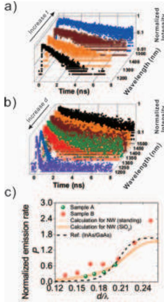
Figure 5. (a,b) Time-resolved emission of Qdisks with variation in (a)  $t$  (sample A) and (b)  $d$  (sample B) inside the single NW on  $\text{SiO}_2$  substrate. (c) Summary of average emission rates. Calculation and reference  $P$  from<sup>18</sup> are shown as orange and black lines, respectively. All measurements were performed using a 80-MHz pulsed laser at 800 nm wavelength and 4K.
