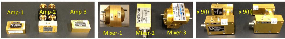
**Fig. 3:** Picture of commercial components used for PM noise measurement at W-band. These are custom components optimized for 92 – 96 GHz.
